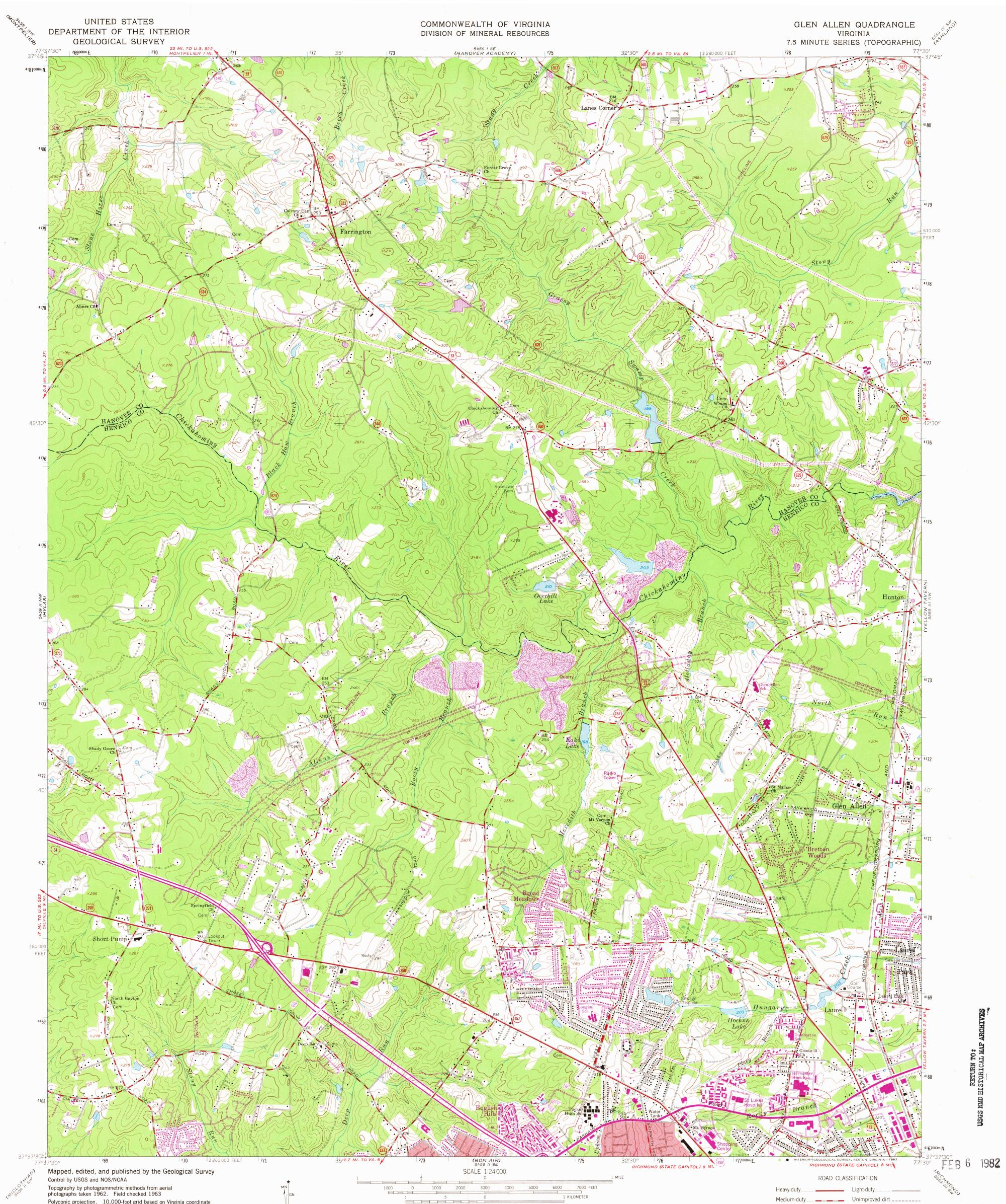
Polyconic projection. 10,000-foot grid based on Virginia coordinate system, south zone. 1000-meter Universal Transverse Mercator grid ticks, zone 18, shown in blue. 1927 North American Datum To place on the predicted North American Datum 1983 move the projection lines 11 meters south and 23 meters west as shown by dashed corner ticks
