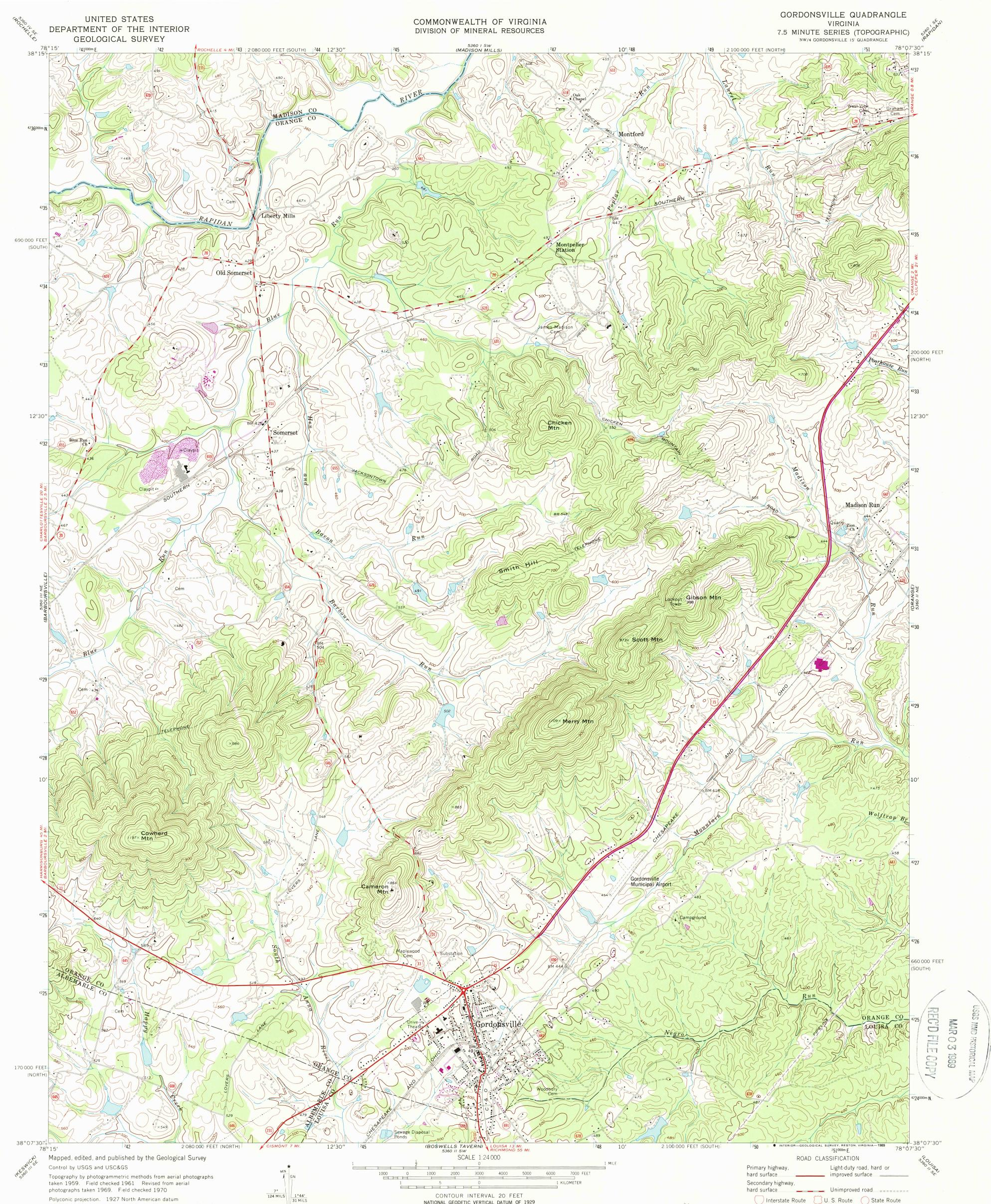
Polyconic projection. 1927 North American datum 10,000-foot grids based on Virginia coordinate system, north and south zones 1000-meter Universal Transverse Mercator grid ticks, zone 17, shown in blue
