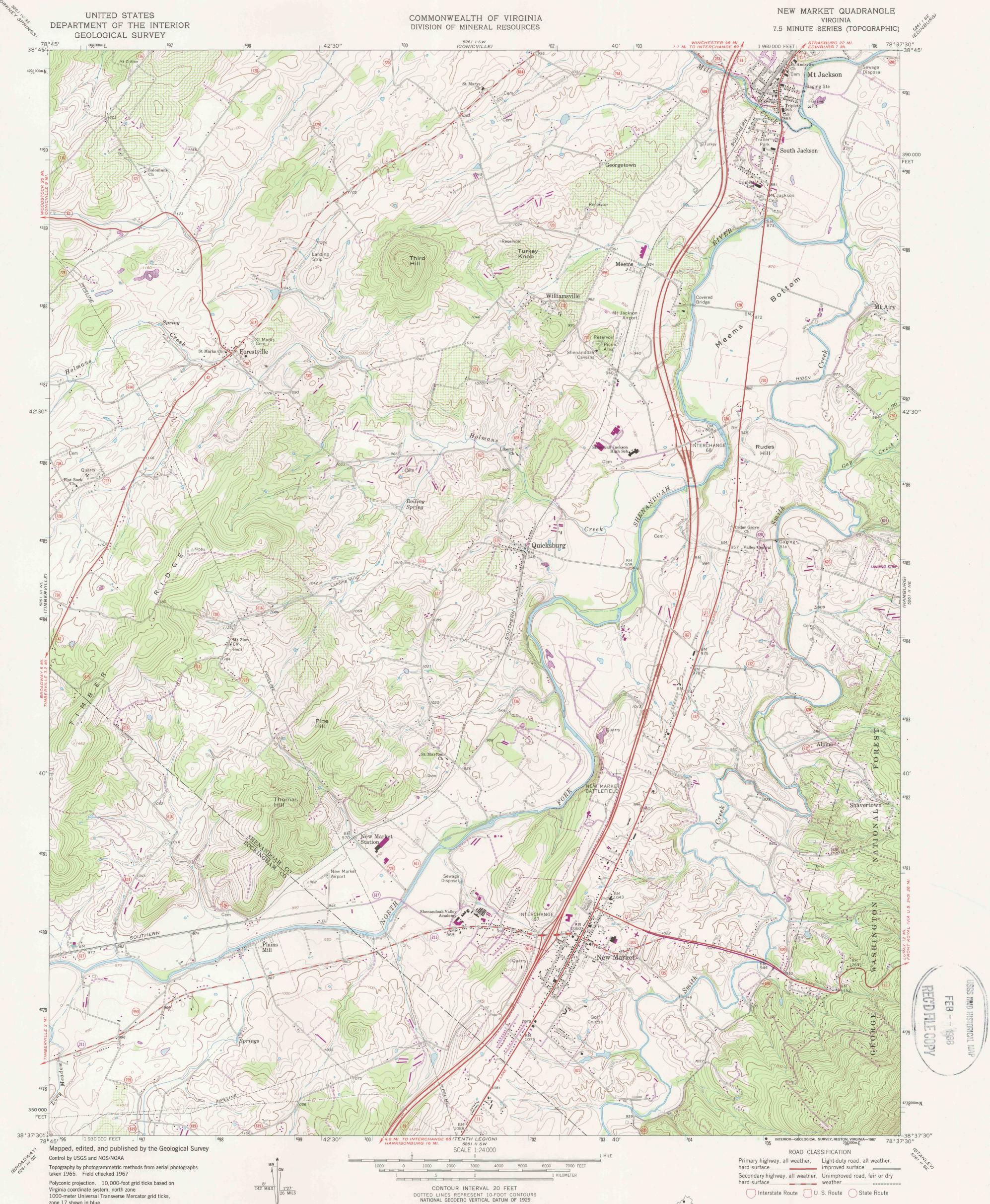
Virginia coordinate system, north zone 1000-meter Universal Transverse Mercator grid ticks, zone 17 shown in blue 1927 North American Datum To place on the predicted North American Datum 1983 move the projection lines 8 meters south and 22 meters west as shown by dashed corner ticks
