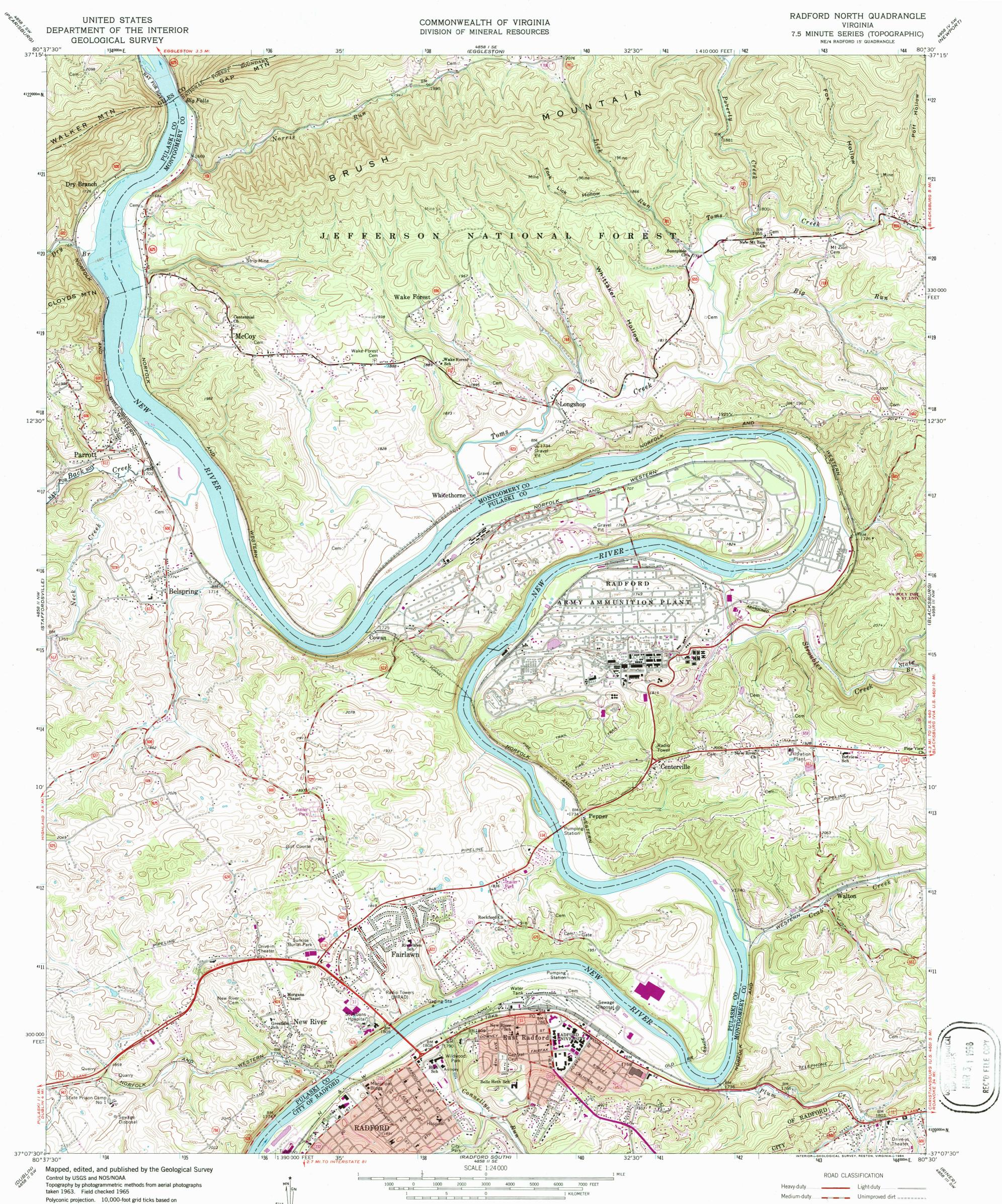
Virginia coordinate system, south zone 1000-meter Universal Transverse Mercator grid ticks, zone 17, shown in blue 1927 North American Datum To place on the predicted North American Datum 1983 move the projection lines 9 meters south and 17 meters west as shown by dashed corner ticks Fine red dashed lines indicate selected fence and field lines where
