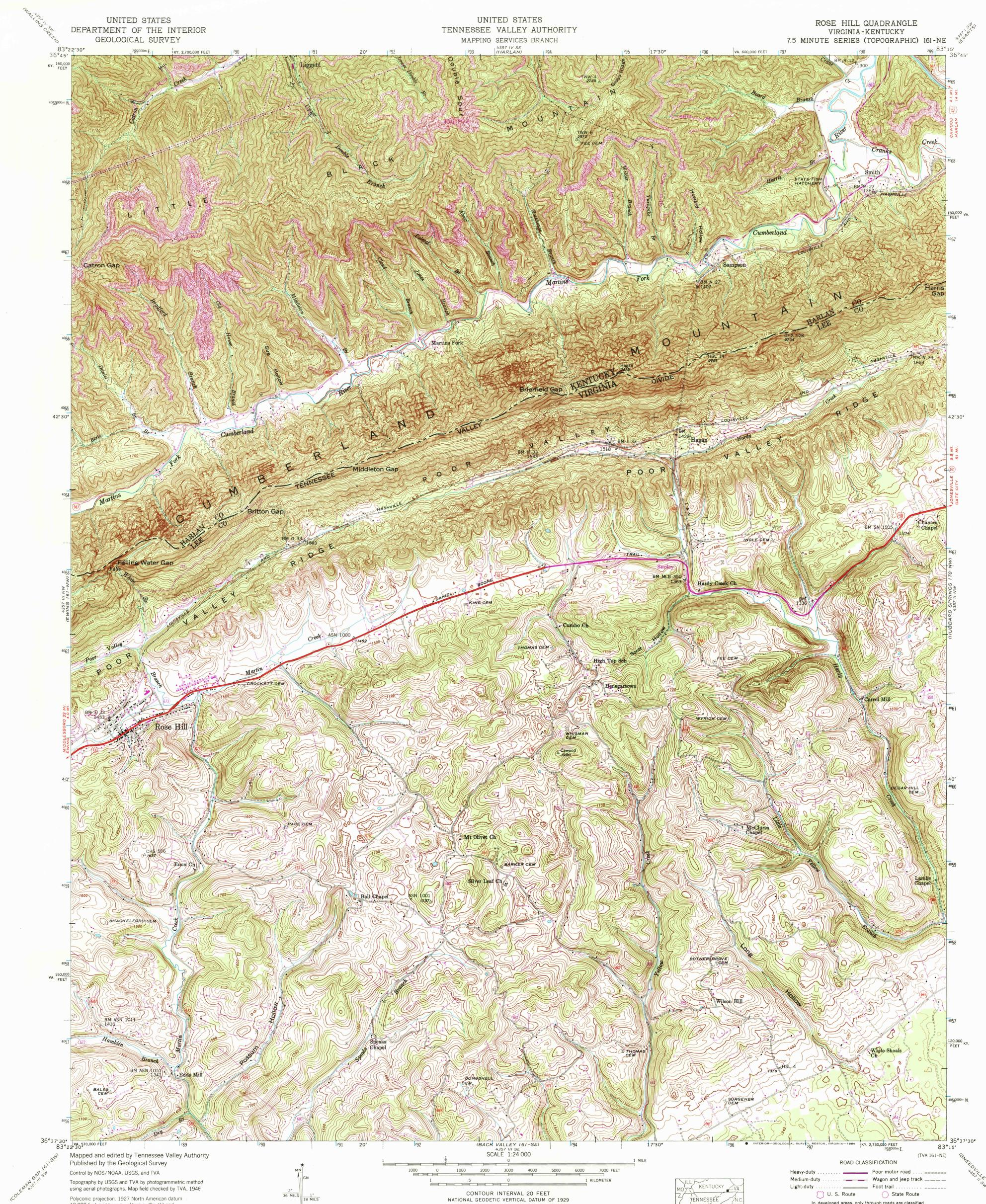
Polyconic projection. 1927 North American datum 10,000 foot grid based on Virginia (South) and Kentucky (South) rectangular coordinate systems 1000 meter Universal Transverse Mercator Grid ticks, Zone 17, shown in blue
