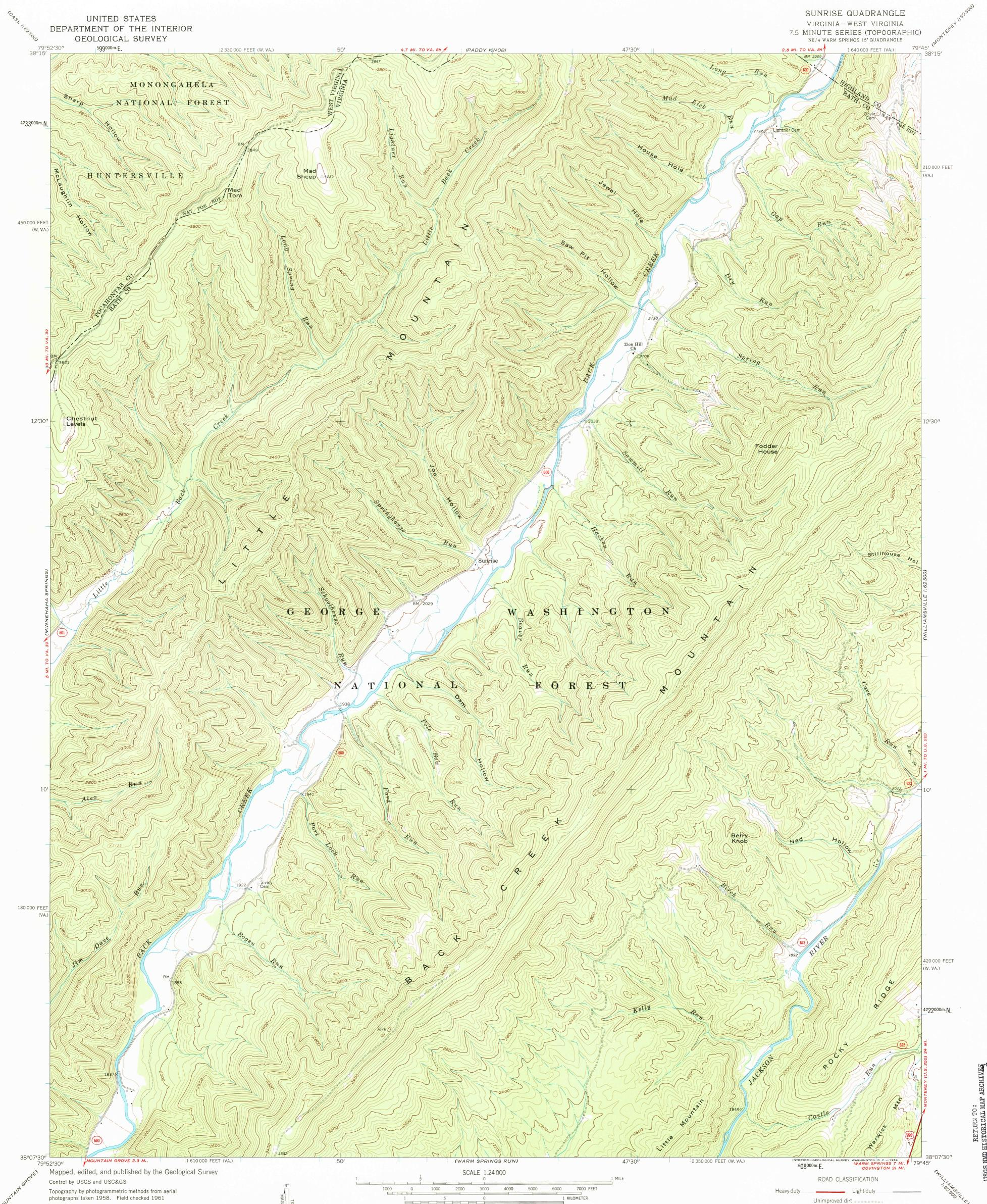
Polyconic projection. 1927 North American datum 10,000-foot grids based on Virginia coordinate system, north zone and West Virginia coordinate system, south zone 1000-meter Universal Transverse Mercator grid ticks, zone 17, shown in blue
