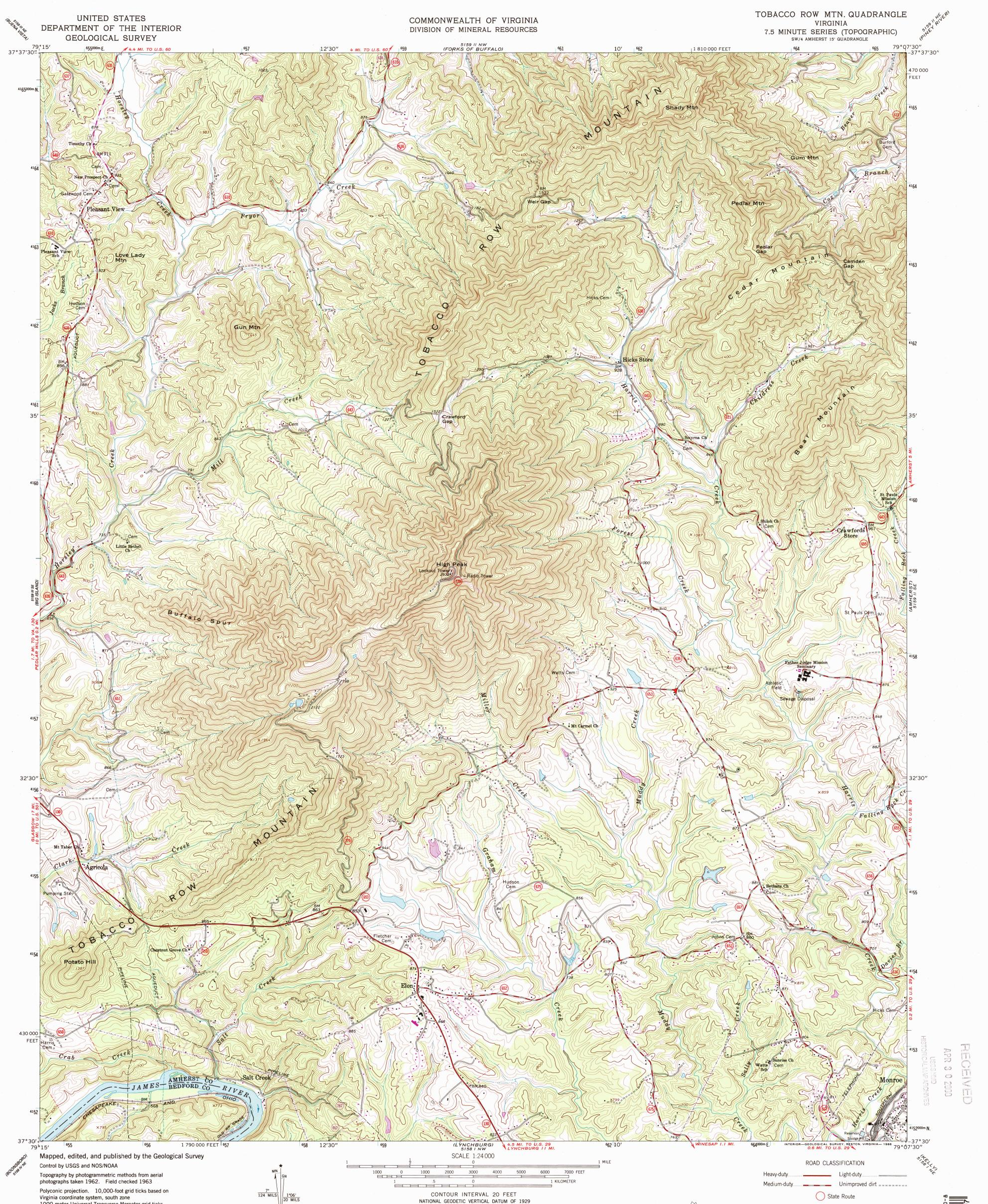
Polyconic projection. 10,000-foot grid ticks based on Virginia coordinate system, south zone 1000-meter Universal Transverse Mercator grid ticks, zone 17, shown in blue 1927 North American Datum To place on the predicted North American Datum 1983 move the projection lines 10 meters south and 22 meters west as shown by dashed corner ticks
