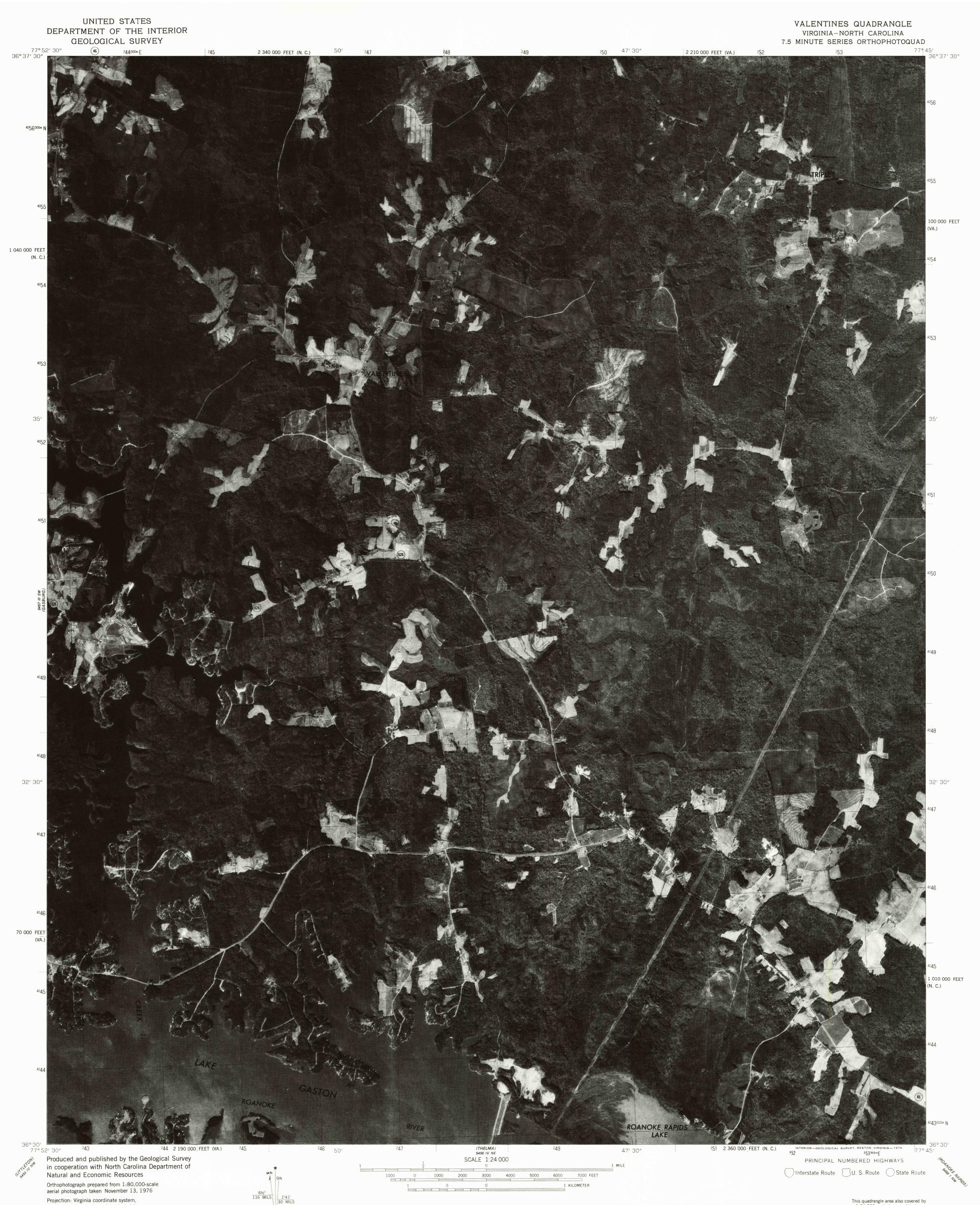
Projection: Virginia coordinate system, south zone (Lambert conformal conic) 10,000-foot grid ticks based on Virginia coordinate system, south zone, and North Carolina coordinate system 1000-meter Universal Transverse Mercator grid, zone 18. 1927 North American datum
