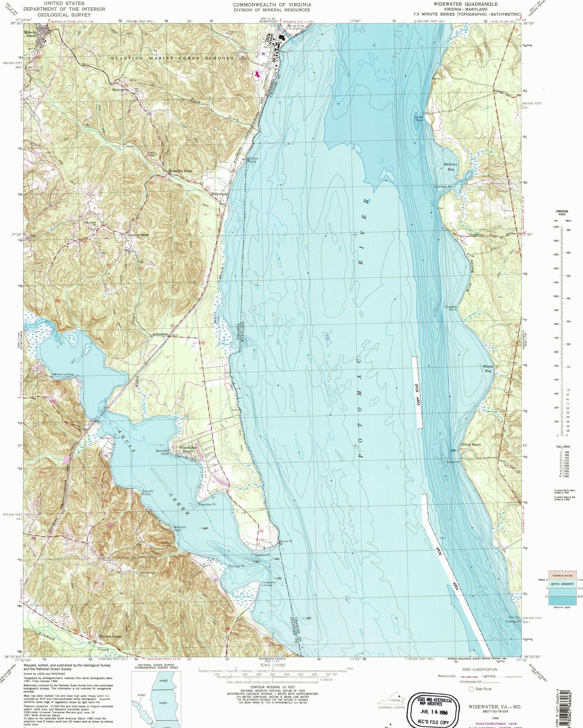
Mean low water (dotted) line and mean high water (heavy solid) line compiled by NOS from tide-coordinated aerial photographs. Apparent shoreline (outer edge of vegetation) shown by light solid line
