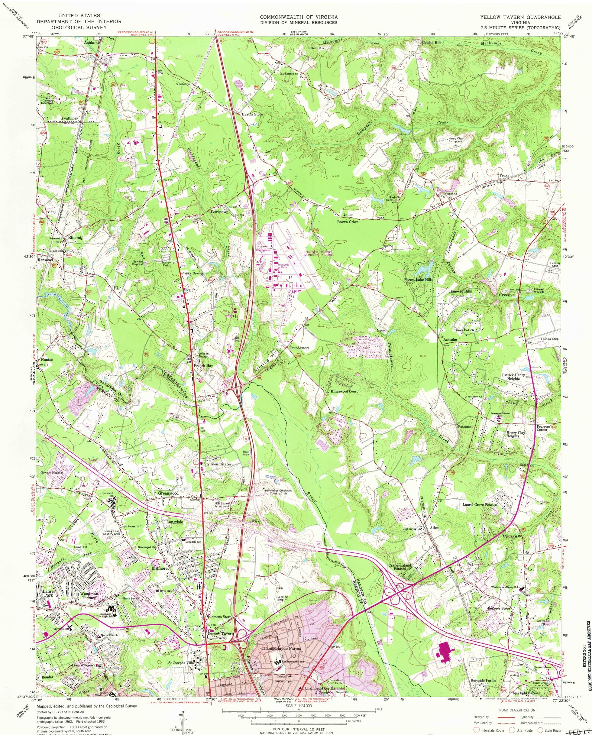
Polyconic projection. 10,000-foot grid based on Virginia coordinate system, south zone 1000-meter Universal Transverse Mercator grid ticks, zone 18, shown in blue. 1927 North American Datum To place on the predicted North American Datum 1983 move the projection lines 10 meters south and 26 meters west as shown by dashed corner ticks
