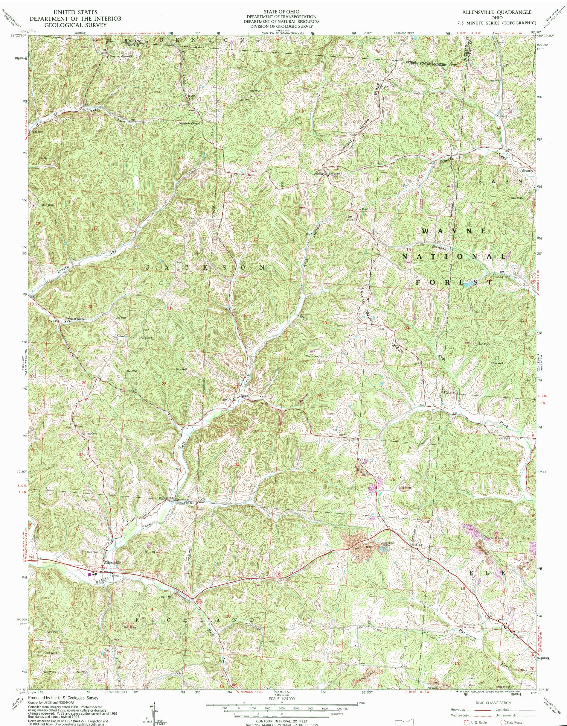
North American Datum of 1927 (NAD 27). Projection and 10 000-foot ticks: Ohio coordinate system, south zone (Lambert conformal conic) Blue 1000-meter Universal Transverse Mercator grid ticks, zone 17 North American Datum of 1983 (NAD 83) is shown by dashed corner ticks. The values of the shift between NAD 27 and NAD 83 for 7.5-minute intersections are obtainable from National Geodetic Survey NADCON software
