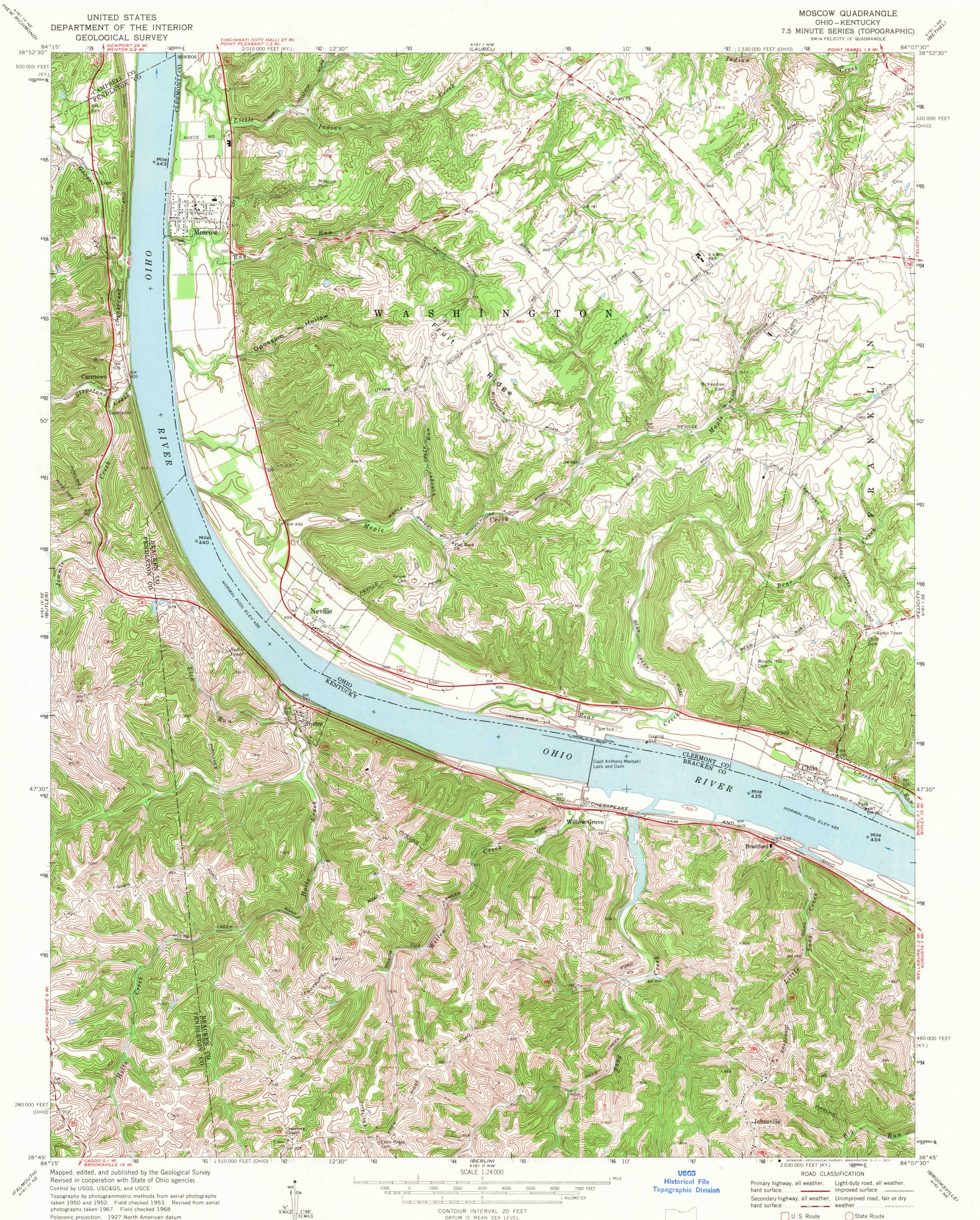
Polyconic projection. 1927 North American datum 10,000-foot grids based on Ohio coordinate system, south zone, and Kentucky coordinate system, north zone 1000-meter Universal Transverse Mercator grid ticks, zone 16, shown in blue
