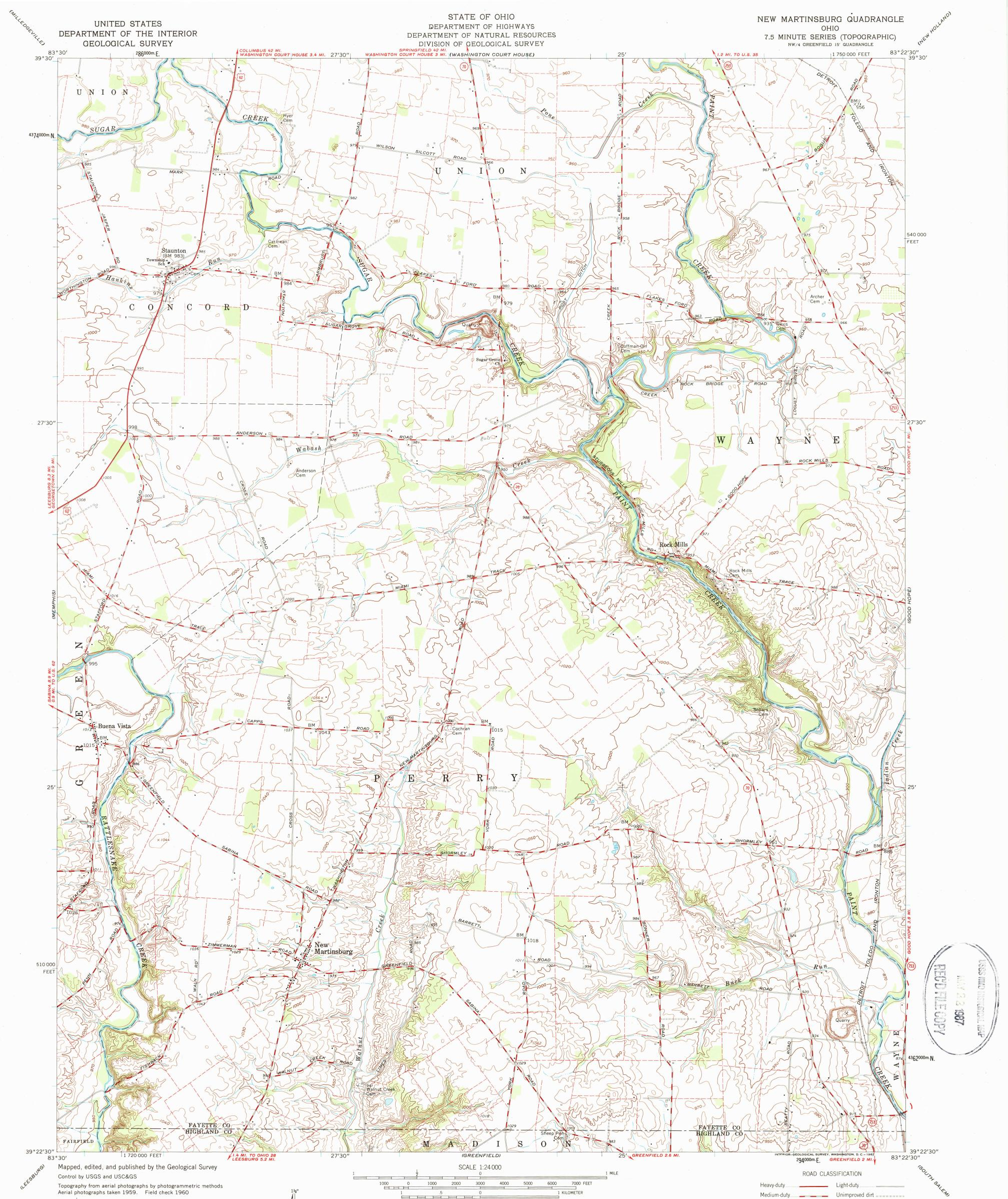
Polyconic projection. 1927 North American datum 10,000-foot grid based on Ohio coordinate system, south zone 1000-meter Universal Transverse Mercator grid ticks, zone 17, shown in blue
