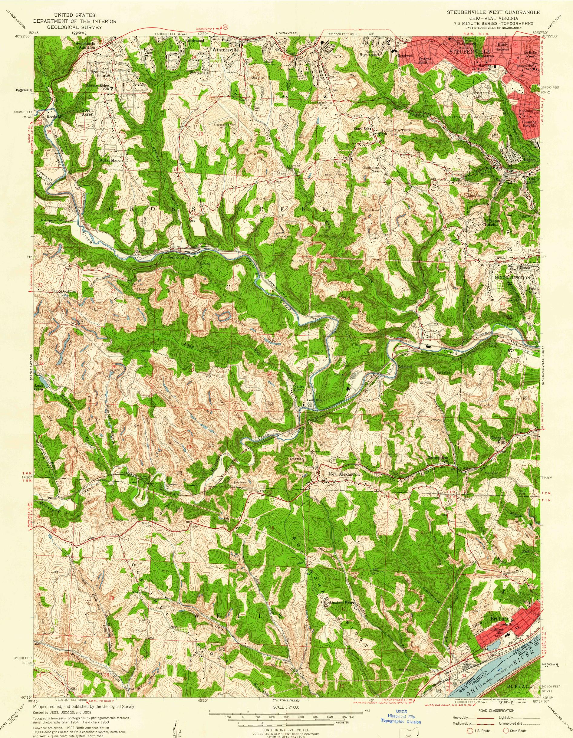
Polyconic projection. 1927 North American datum 10,000-foot grids based on Ohio coordinate system, north zone, and West Virginia coordinate system, north zone 1000-meter Universal Transverse Mercator grid ticks, zone 17, shown in blue
