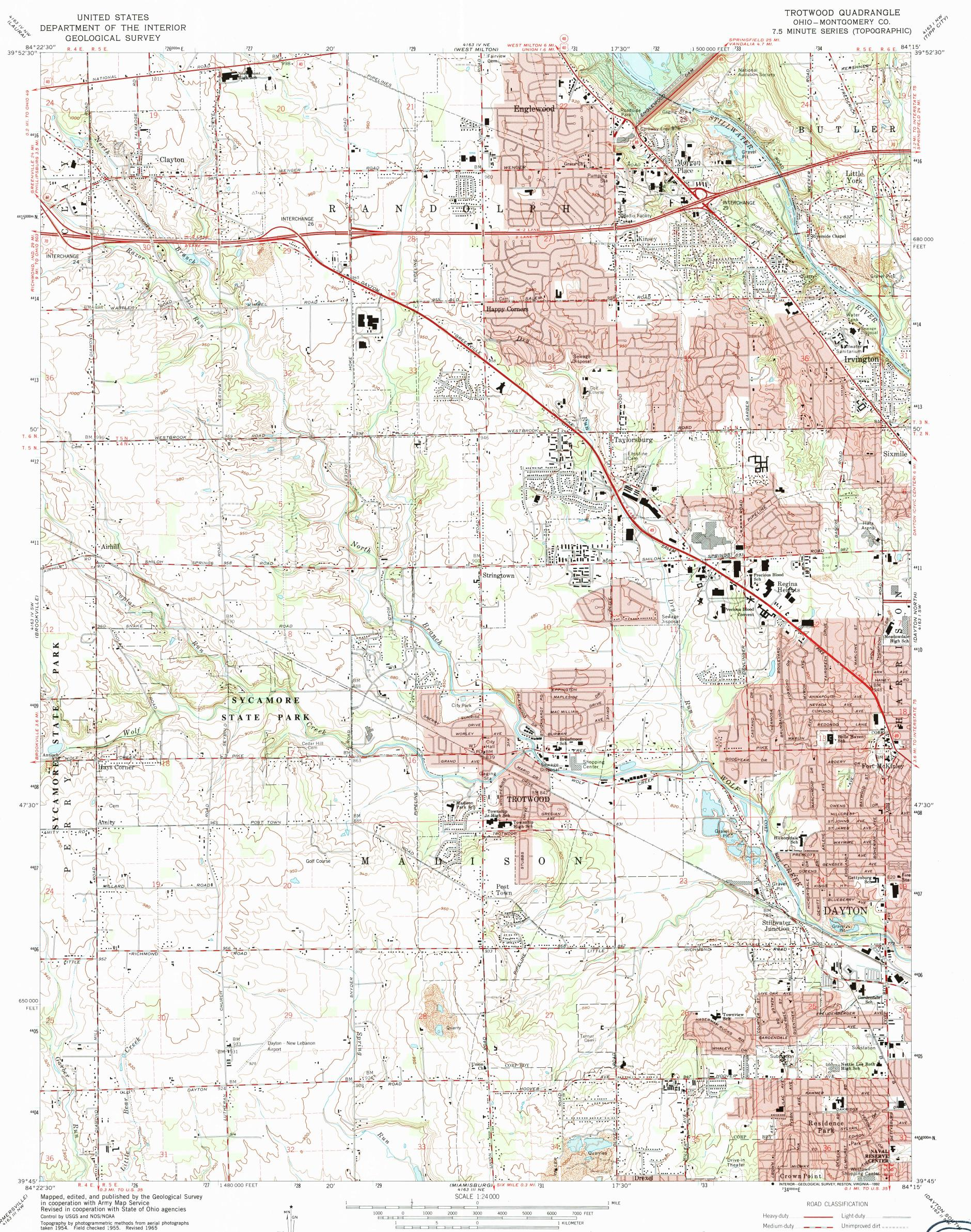
Polyconic projection. 10,000-foot grid ticks based on Ohio coordinate system, south zone. 1000-meter Universal Transverse Mercator grid ticks, zone 16, shown in blue. 1927 North American Datum. The difference between 1927 North American Datum and North American Datum of 1983 (NAD 83) for 7.5-minute intersections is given in USGS Bulletin 1875. The NAD 83 is shown by
