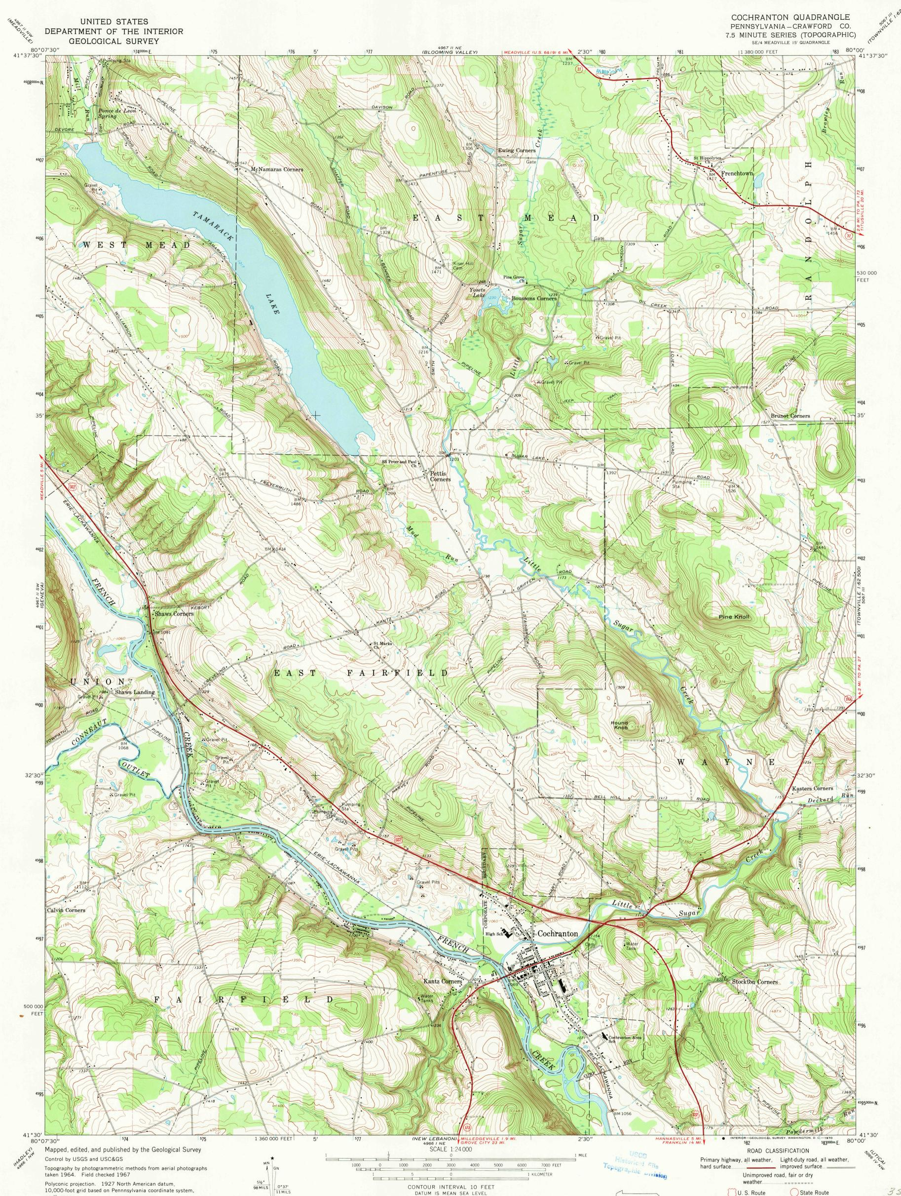
Polyconic projection. 1927 North American datum. 10,000-foot grid based on Pennnsylvania coordinate system, north zone 1000-meter Universal Transverse Mercator grid ticks, zone 17, shown in blue
