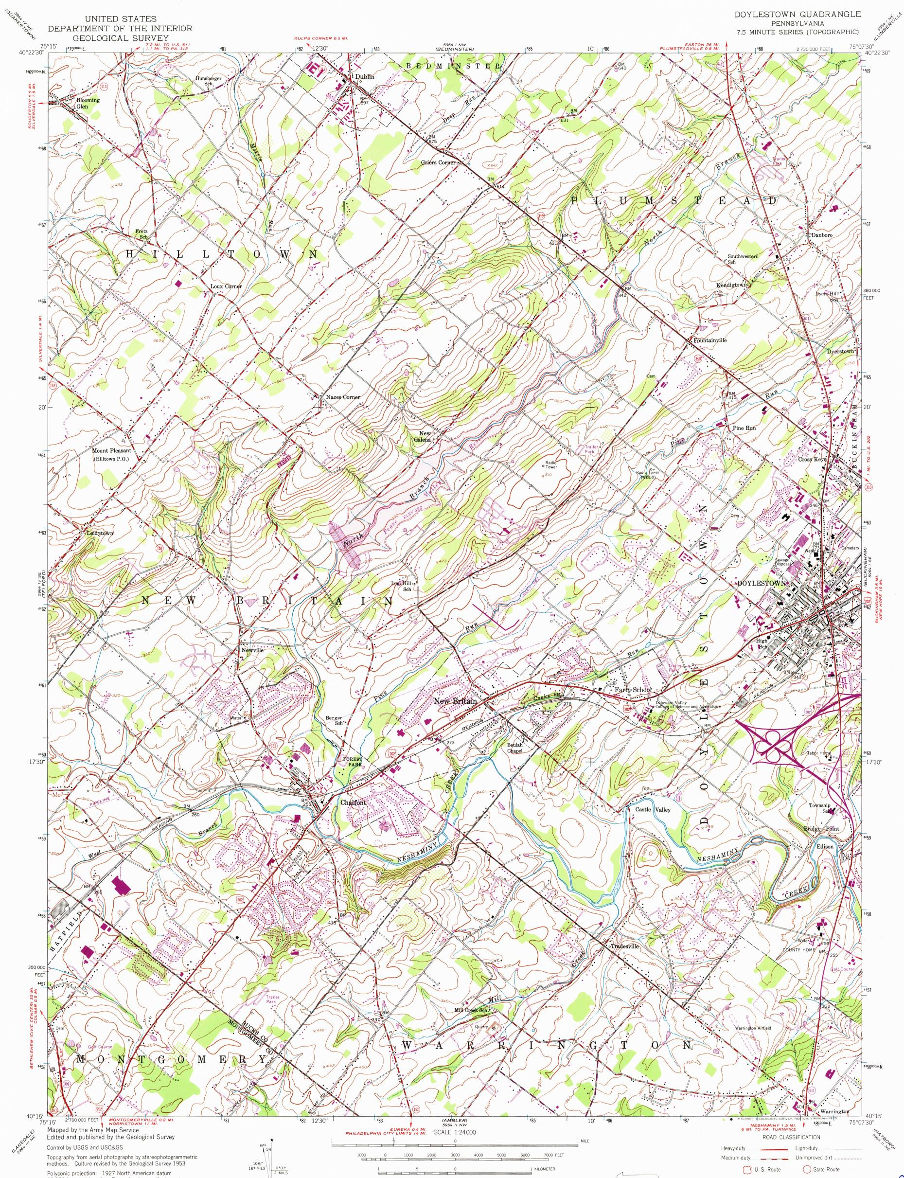
Polyconic projection. 1927 North American datum 10,000-foot grid based on Pennsylvania coordinate system, south zone 1000-meter Universal Transverse Mercator grid ticks, zone 18, shown in blue Purple hatching indicates areas to be submerged
