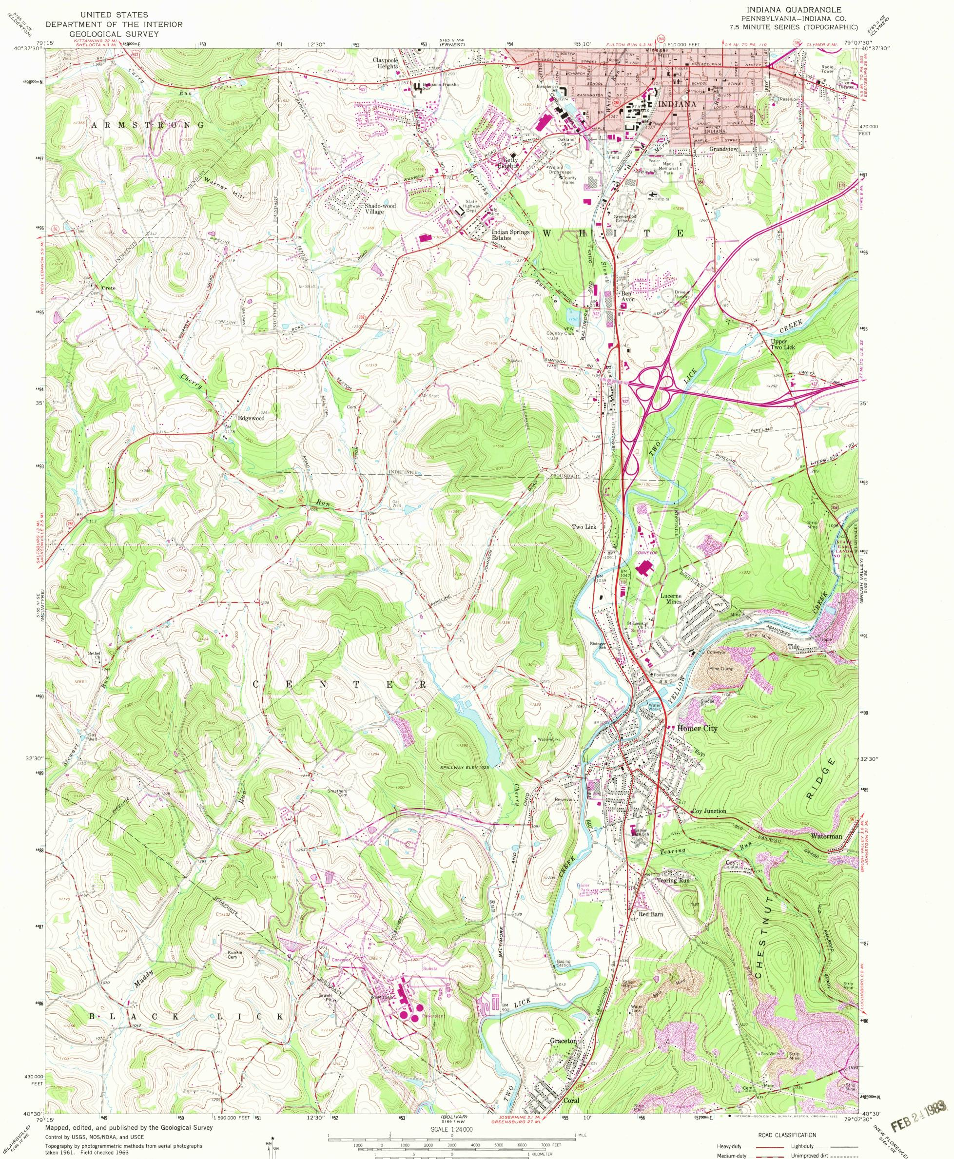
Polyconic projection. 10,000-foot grid ticks based on Pennsylvania coordinate system, south zone. 1000-meter Universal Transverse Mercator grid ticks, zone 17, shown in blue. 1927 North American Datum. To place on the predicted North American Datum 1983 move the projection lines 4 meters south and 20 meters west as shown by dashed corner ticks Fine red dashed lines indicate selected fence and field lines where
