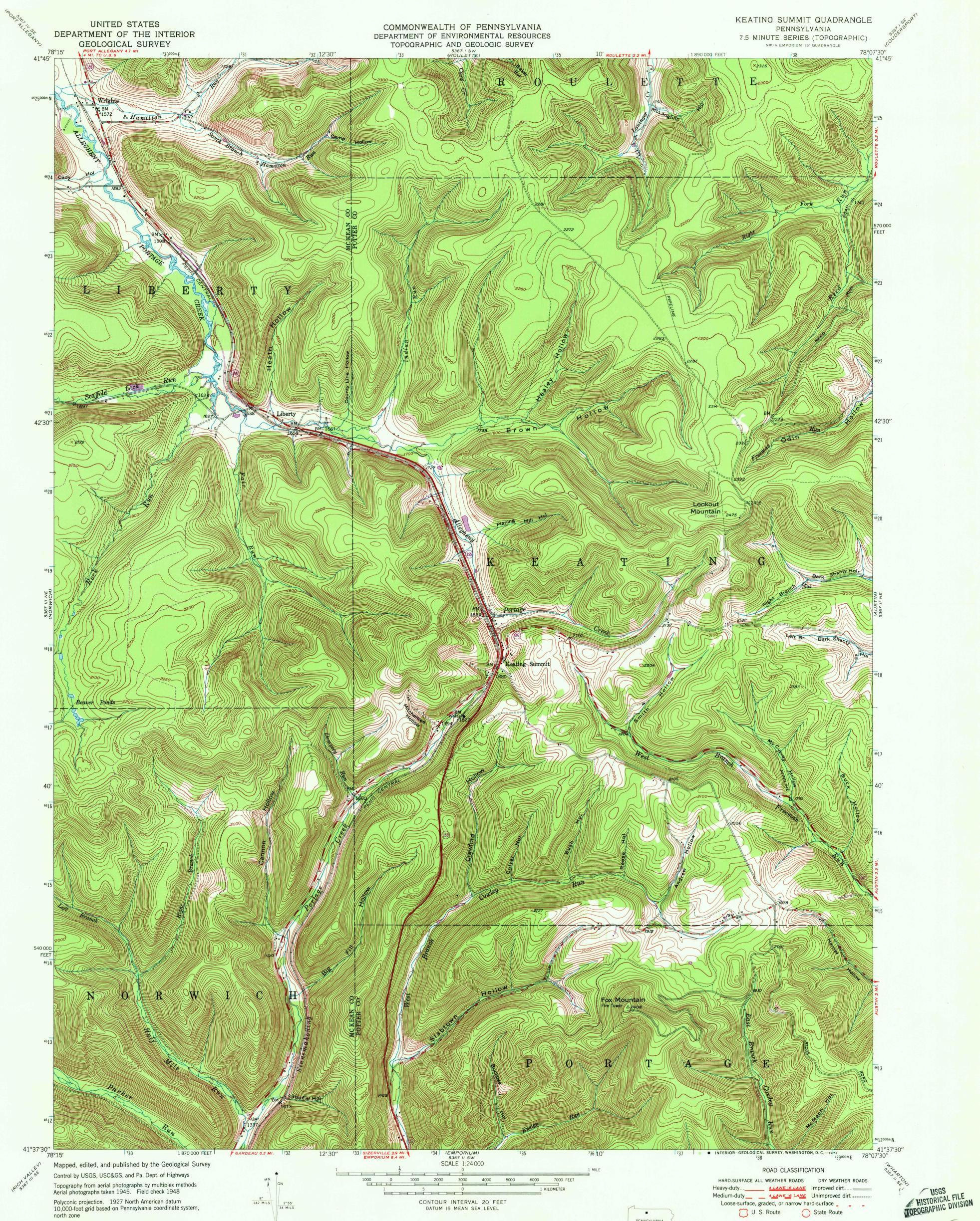
Polyconic projection. 1927 North American datum 10,000-foot grid based on Pennsylvania coordinate system, north zone
