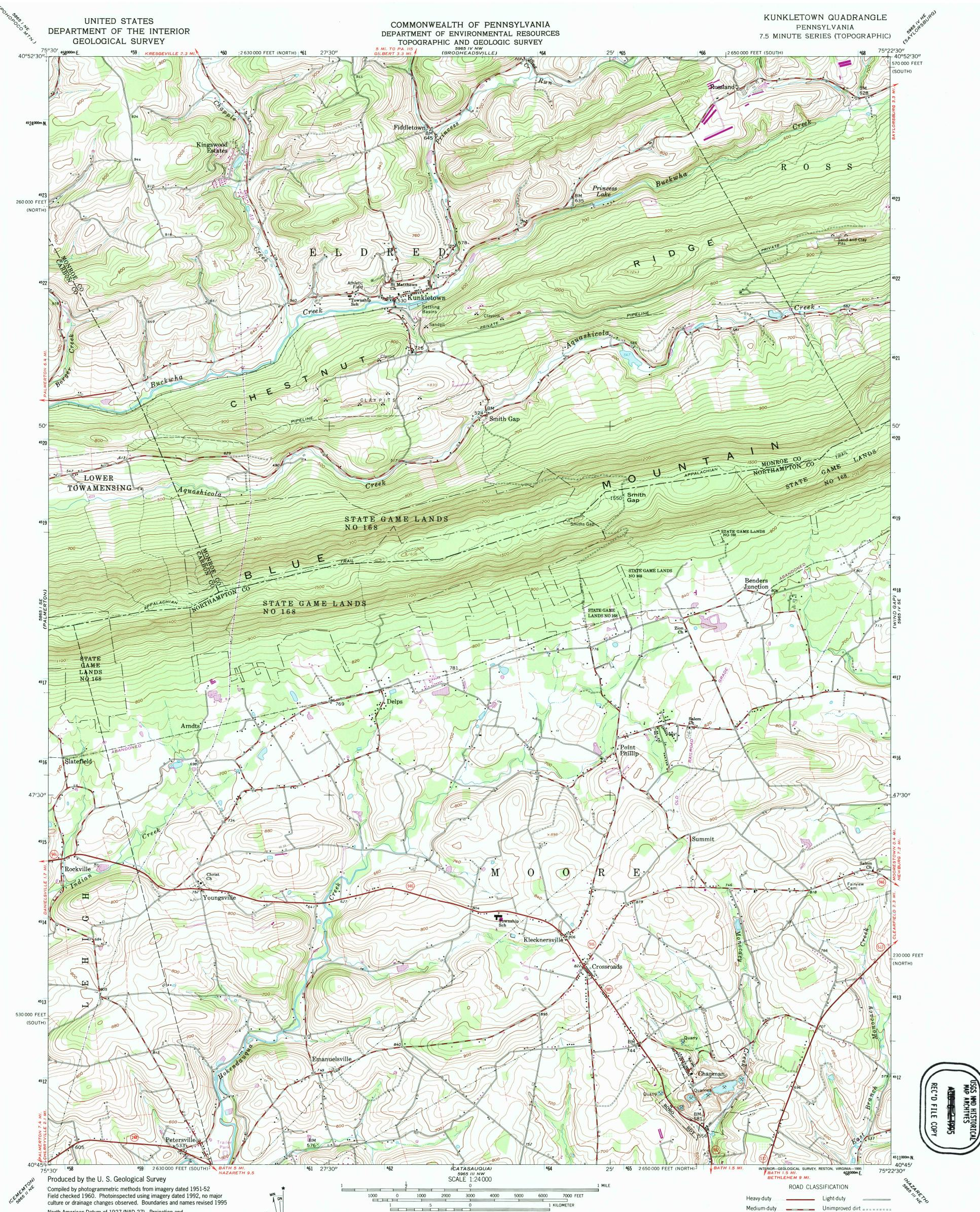
North American Datum of 1927 (NAD 27). Projection and 10 000-foot ticks: Pennsylvania coordinate system, south and north zones (Lambert conformal conic) Blue 1000-meter Universal Transverse Mercator grid ticks, zone 18
