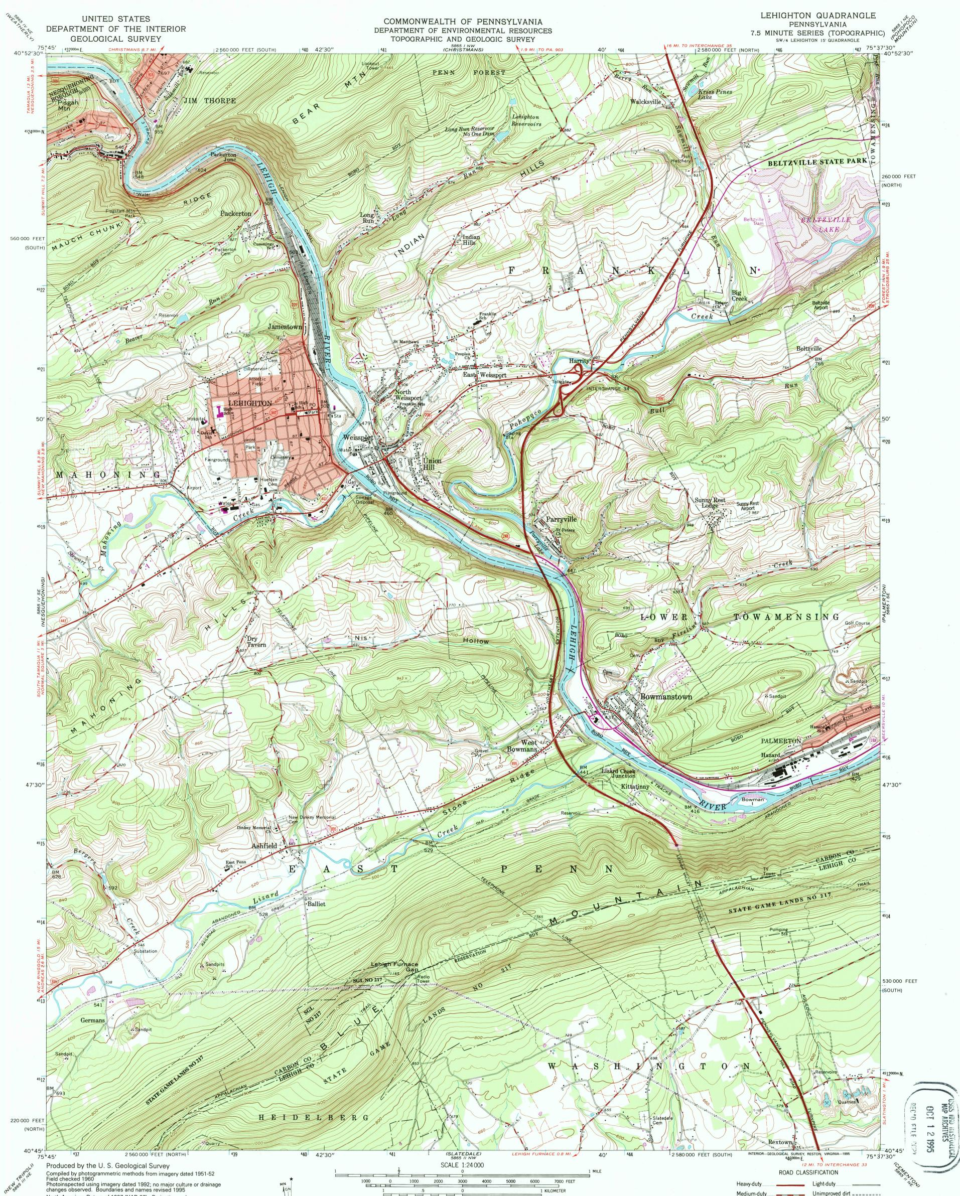
North American Datum of 1927 (NAD 27). Projection and 10 000-foot ticks: Pennsylvania coordinate system, north and south zones (Lambert conformal conic) Blue 1000-meter Universal Transverse Mercator grid ticks, zone 18 North American Datum of 1983 (NAD 83) is shown by dashed corner ticks. The values of the shift between NAD 27 and NAD 83 for 7.5-minute intersections are obtainable from National Geodetic Survey NADCON software
