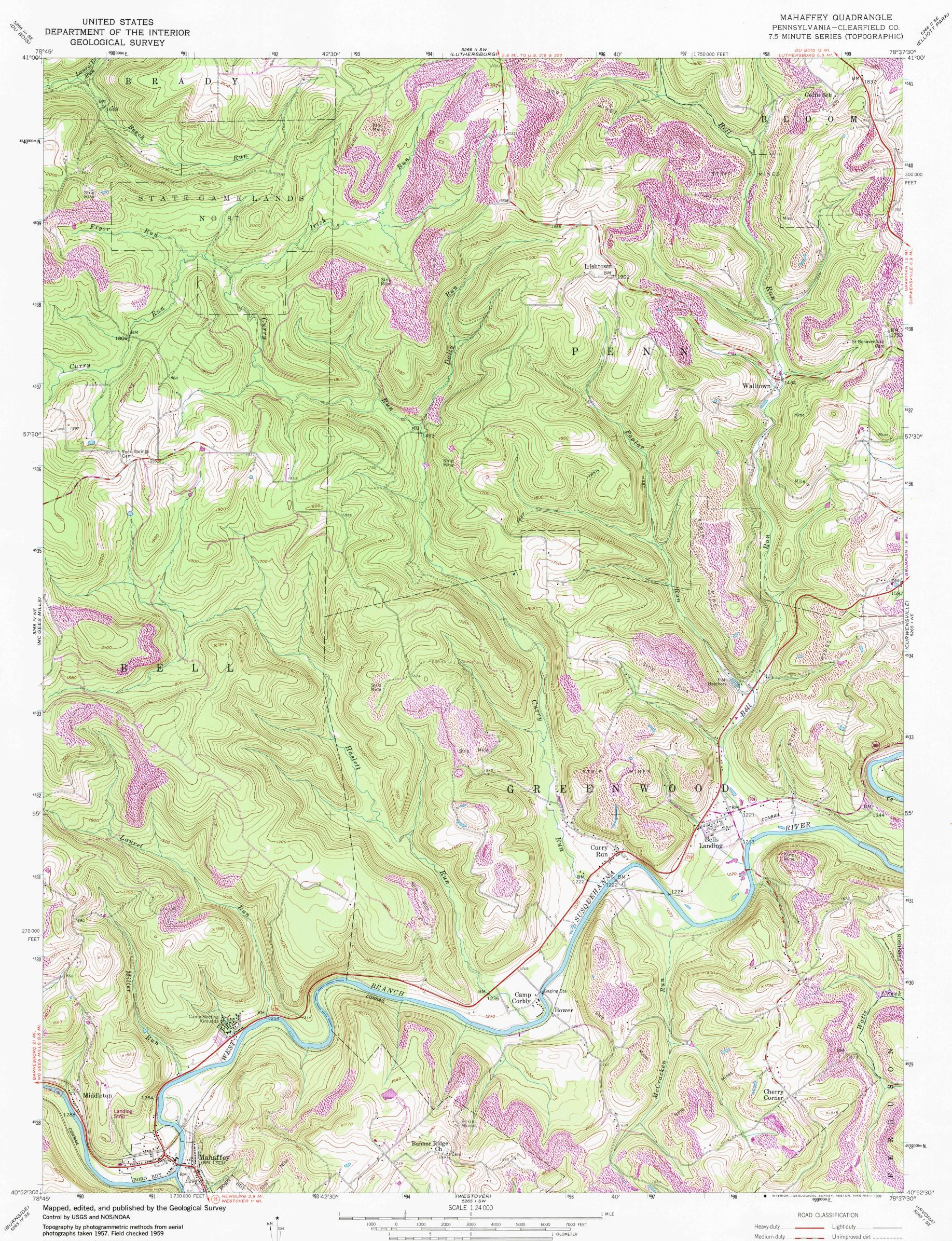
Polyconic projection. 10,000-foot grid ticks based on Pennsylvania coordinate system, north zone 1000-meter Universal Transverse Mercator grid ticks, zone 17, shown in blue. 1927 North American Datum To place on the predicted North American Datum 1983 move the projection lines 4 meters south and 22 meters west as shown by dashed corner ticks UTM GRID AND 1981 MAGNETIC NORTH DECLINATION AT CENTER OF SHEET
