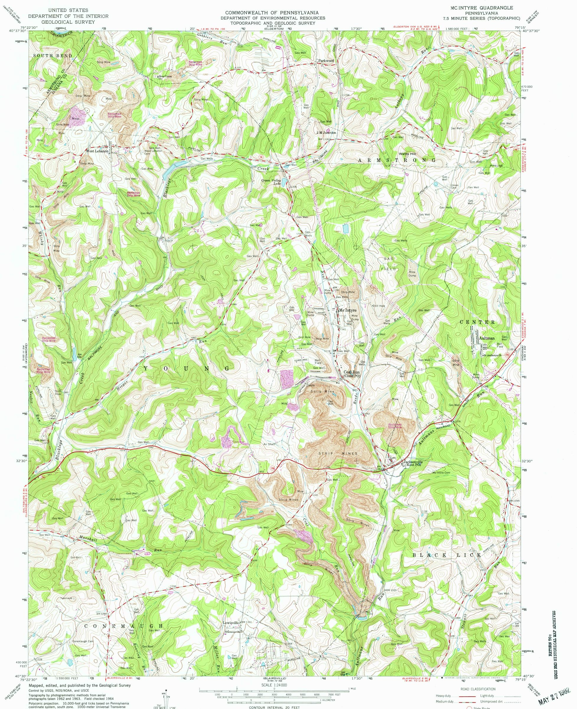
Polyconic projection. 10,000-foot grid ticks based on Pennsylvania coordinate system, south zone. 1000-meter Universal Transverse Mercator grid ticks, zone 17, shown in blue. 1927 North American Datum. To place on the predicted North American Datum 1983 move the projection lines 4 meters south and 20 meters west as shown by dashed corner ticks
