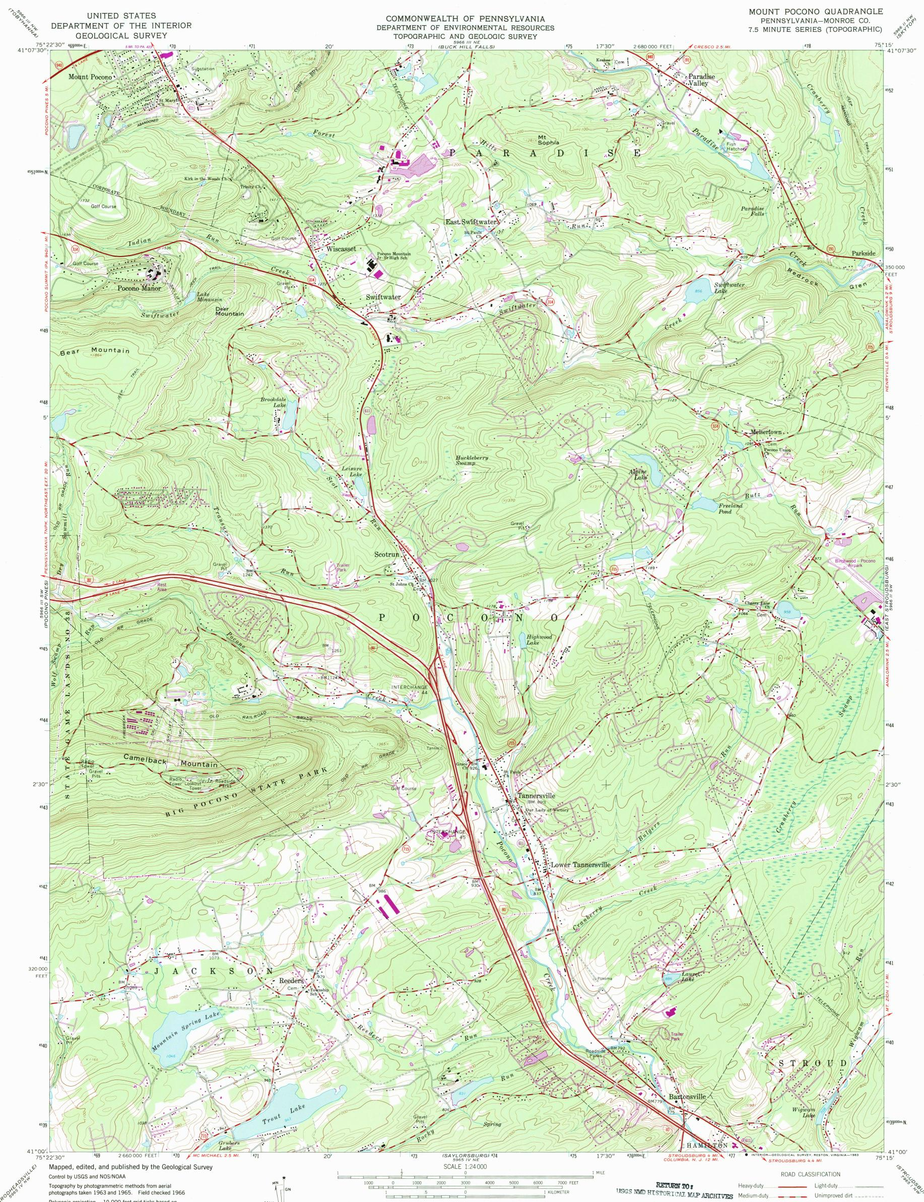
Polyconic projection. 10,000-foot grid ticks based on Pennsylvania coordinate system, north zone 1000-meter Universal Transverse Mercator grid ticks, zone 18, shown in blue. 1927 North American Datum To place on the predicted North American Datum 1983 move the projection lines 6 meters south and 31 meters west as shown by dashed corner ticks  $\frac{11\frac{12}{204}}{204}$   $\frac{0^{\circ}12'}{4}$   $\frac{1}{4}$   $\frac{1}$
