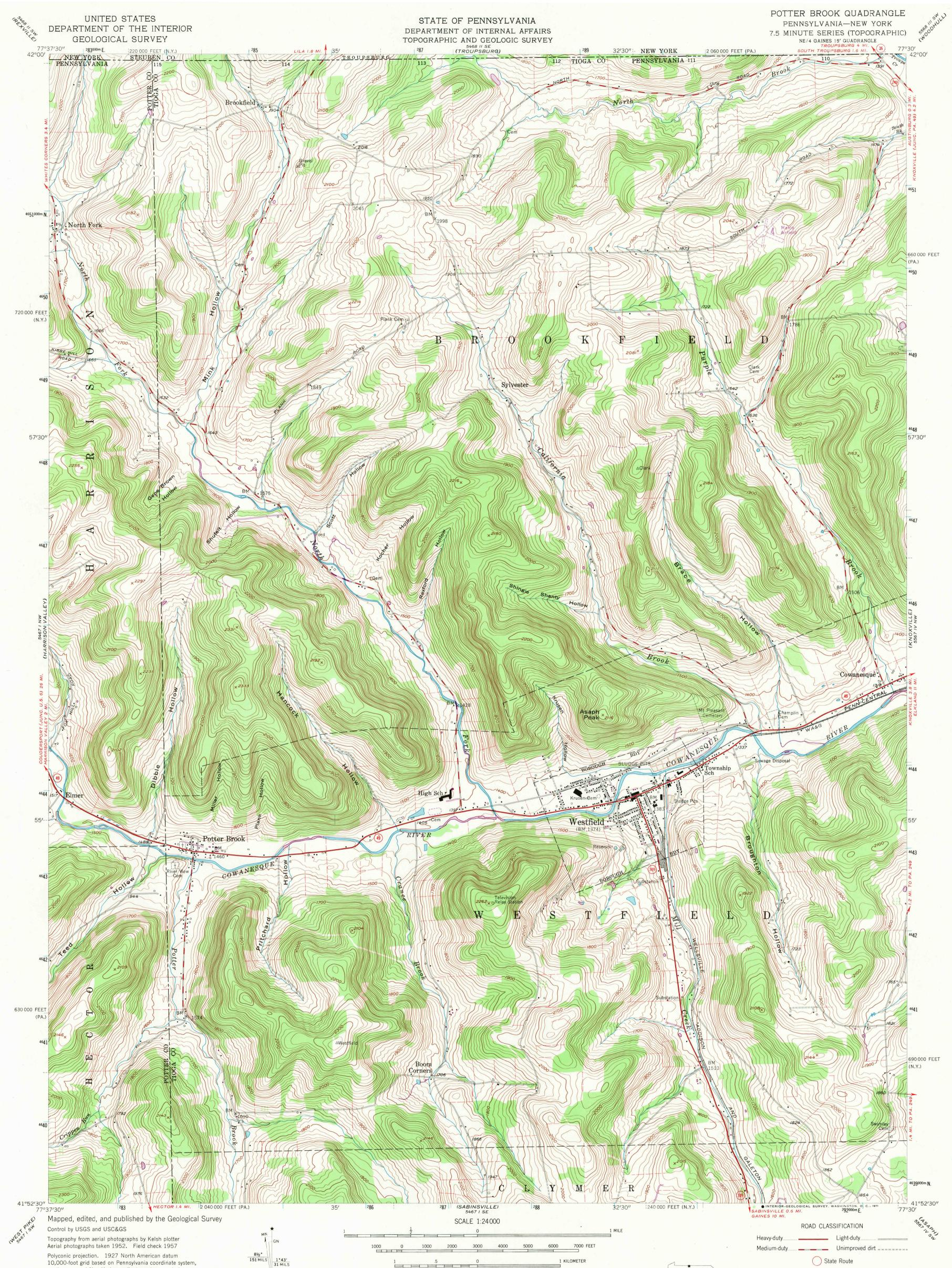
10,000-foot grid based on Pennsylvania coordinate system, north zone, and New York coordinate system, central zone 1000-meter Universal Transverse Mercator grid ticks, zone 18, shown in blue
