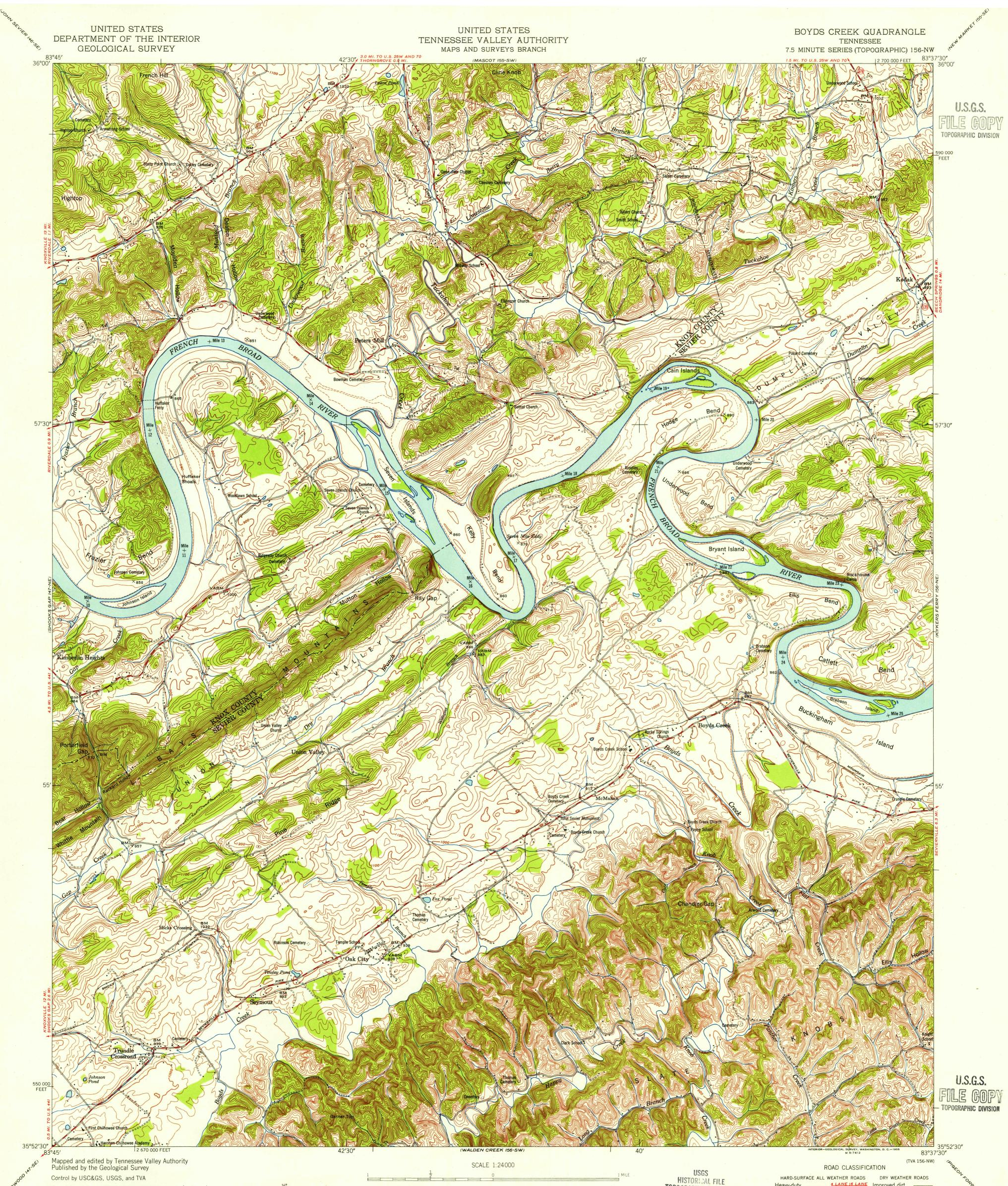
Complete revision by TVA 1952 by photogrammetric (multiplex) methods using aerial photographs taken 1952 and by reference to TVA-USGS quadrangle dated 1940. Original map compiled by photogrammetric (multiplex) methods from aerial photographs taken 1939. Map field checked by TVA 1953.
