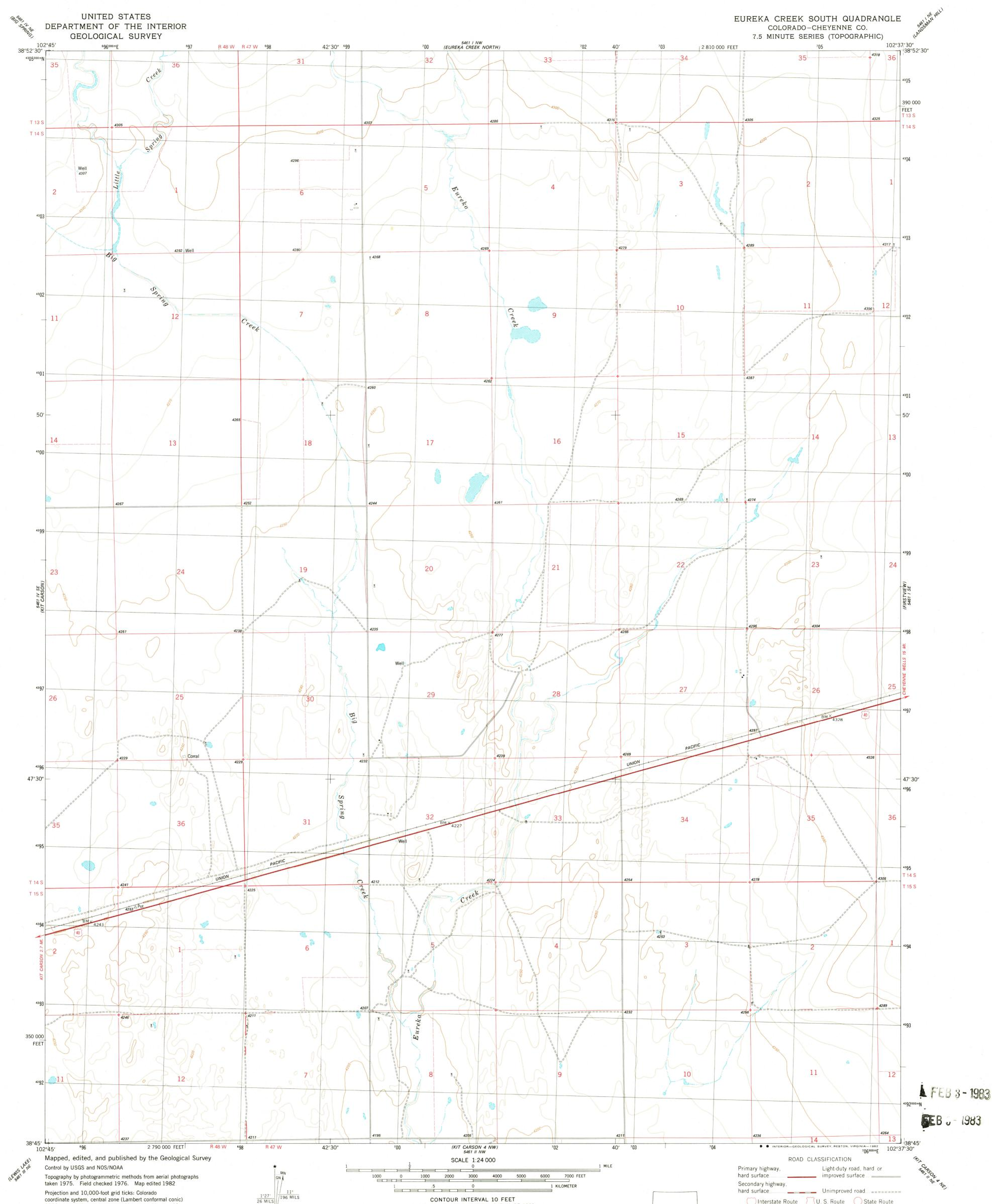
coordinate system, central zone (Lambert conformal conic) 1000-meter Universal Transverse Mercator grid, zone 13 1927 North American datum To place on the predicted North American Datum 1983 move the projection lines 3 meters north and 42 meters east as shown by dashed corner ticks
