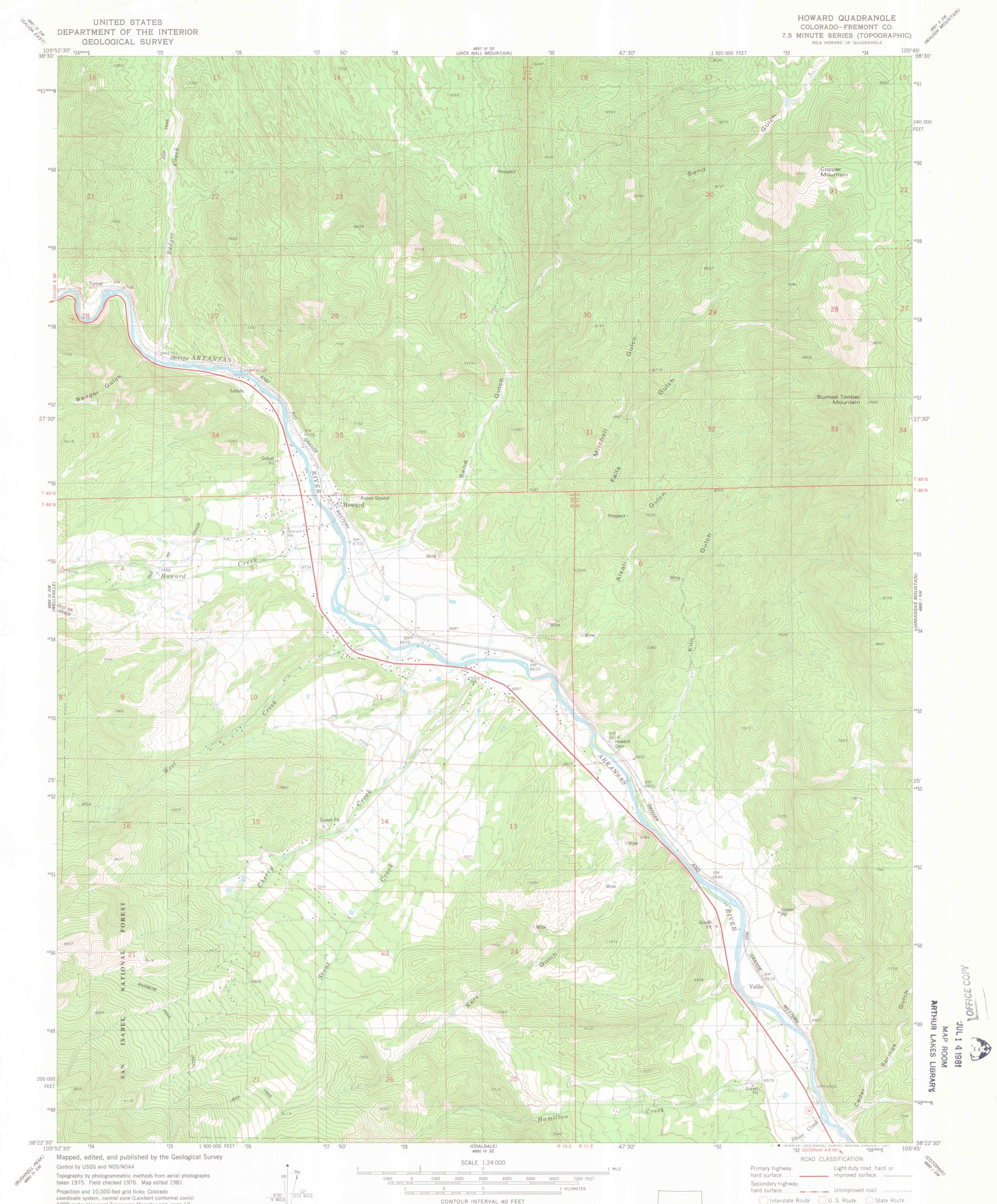
coordinate system, central zone (Lambert conformal conic) 1000-meter Universal Transverse Mercator grid, zone 13 1927 North American datum To place on the predicted North American Datum 1983 move the projection lines 4 meters north and 50 meters east as shown by dashed corner ticks Fine red dashed lines indicate selected fence lines Certain land lines are omitted because of insufficient data
