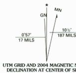
UTM GRID AND 2004 MAGNETIC NORTH DECLINATION AT CENTER OF SHEET
