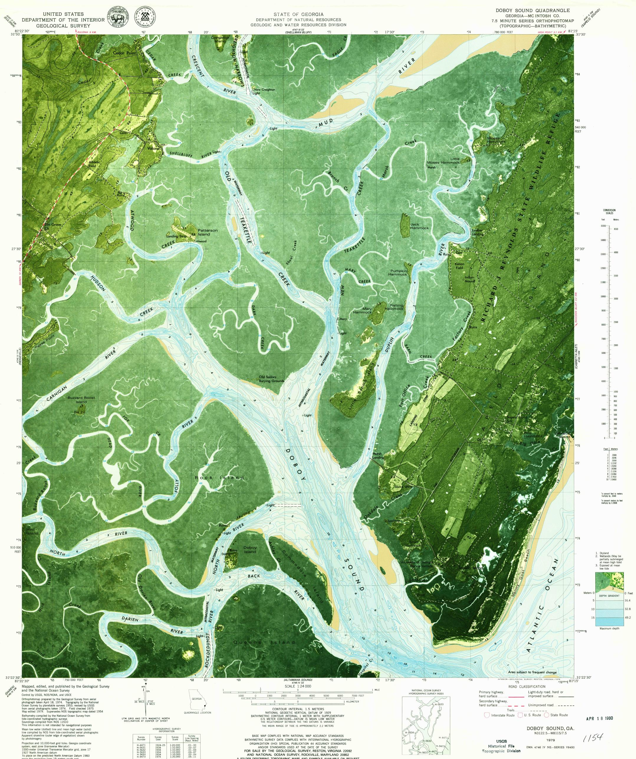
1000-meter Universal Transverse Mercator grid, zone 17 1927 North American datum To place on the predicted North American Datum 1983 move the projection lines 19 meters south and 17 meters west as shown by dashed corner ticks
