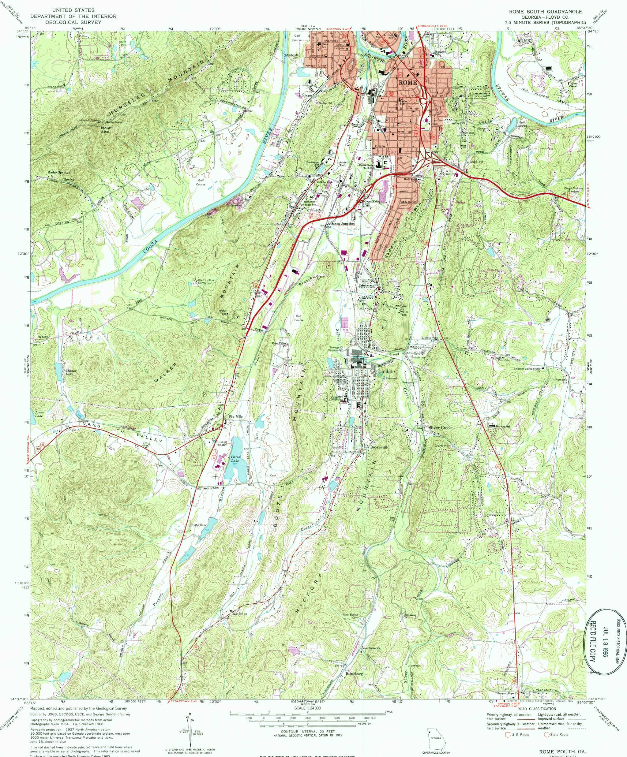
To place on the predicted North American Datum 1983, move the projection lines 9 meters south and 5 meters west as shown by dashed corner ticks
