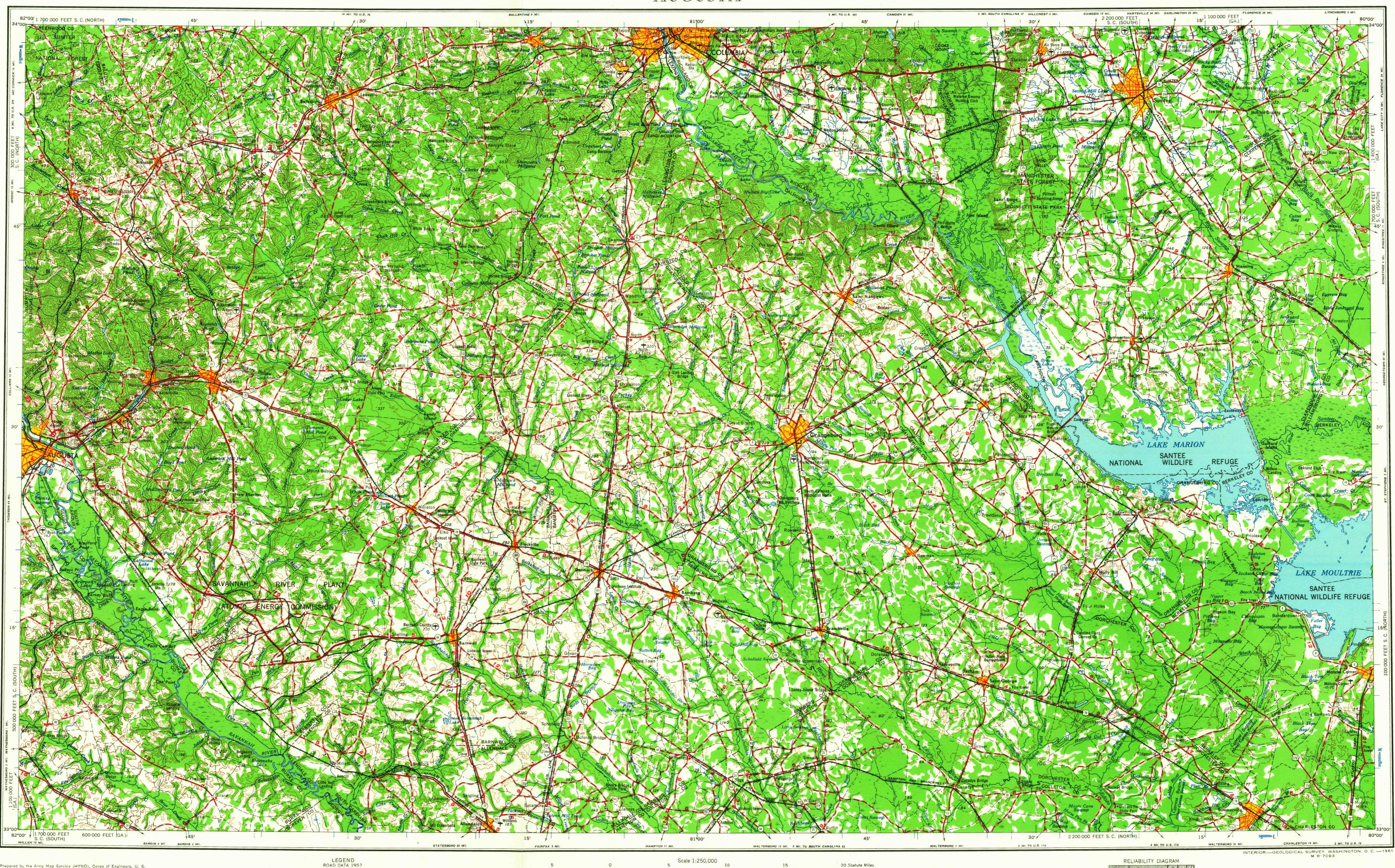
Prepared by the Army Map Service (HYND), Corps of Engineers, U. S. Army, Washington, D. C. Compiled in 1957 by photogrammetric methods and from: United States Quadrangles, 1:25,000 and 1:50,000, CE, 1918-43. Planimetric detail revised by photo-planimetric methods. Horizontal and vertical control by USC&GS, USGS and TVA. Map field checked 1957.
