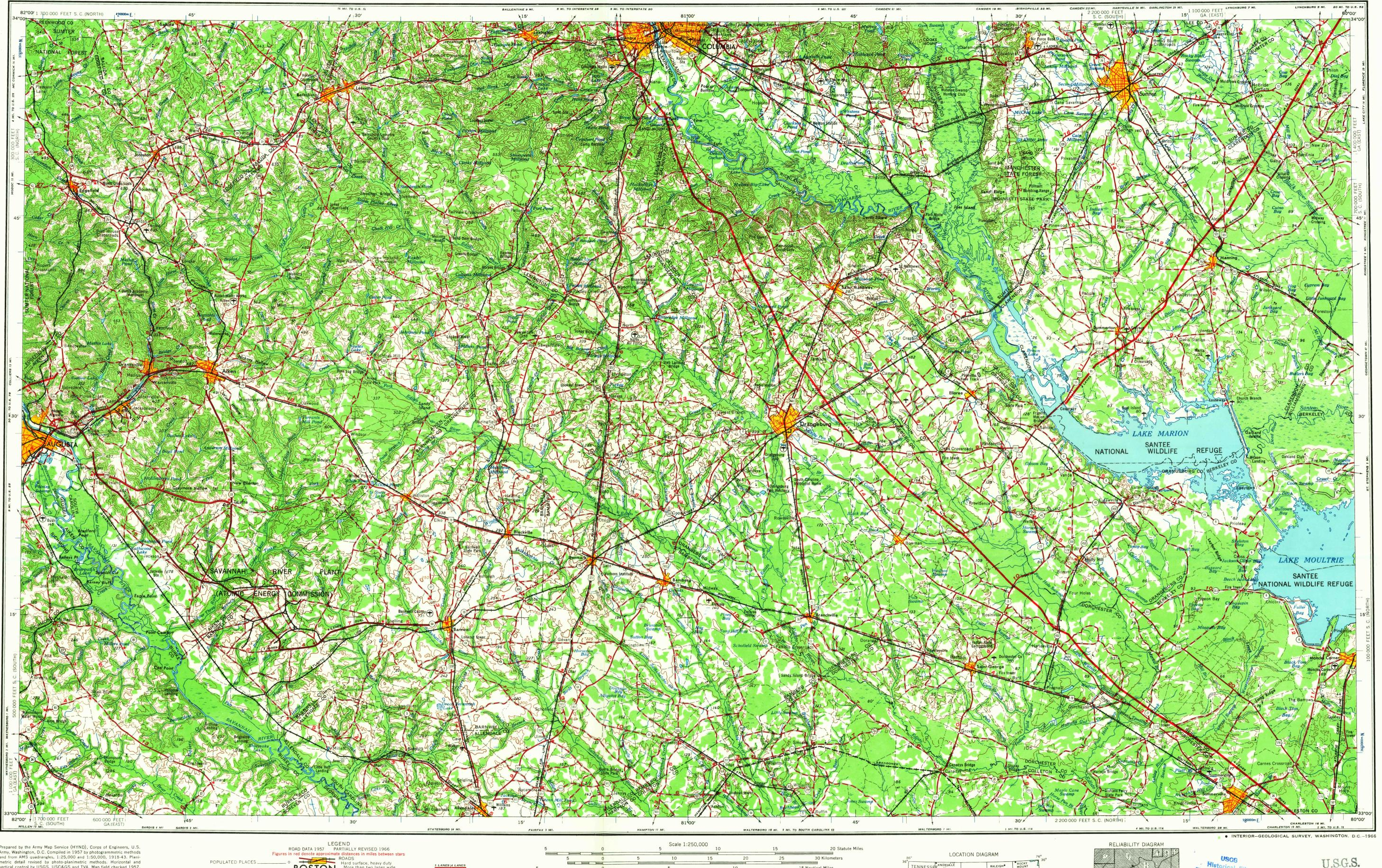
Prepared by the Army Map Service (HYND), Corps of Engineers, U.S. Army, Washington, D.C. Compiled in 1957 by photogrammetric methods and from AMS quadrangles, 1:25,000 and 1:50,000, 1918-43. Planimetric detail revised by photo-planimetric methods. Horizontal and vertical control by USGS, USC&GS and TVA. Map field checked 1957. Limited revision by U.S. Geological Survey 1966.
