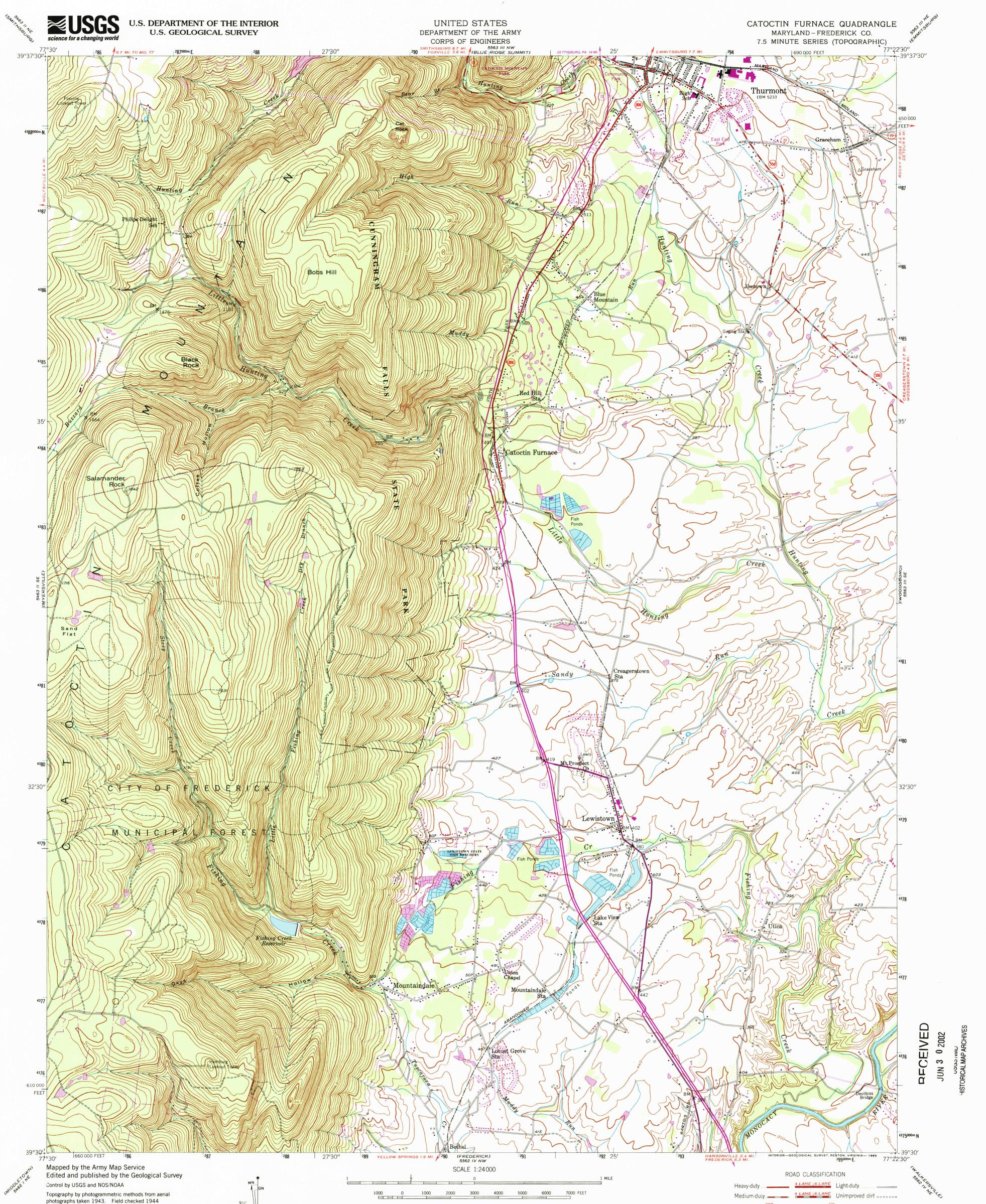
Culture revised by the Geological Survey 1953 Polyconic projection. 10,000-foot grid ticks based on Maryland coordinate system 1000-meter Universal Transverse Mercator grid ticks, zone 18, shown in blue 1927 North American Datum To place on the predicted North American Datum 1983 move the projection lines 7 meters south and 25 meters west as shown by dashed corner ticks There may be private inholdings within the boundaries of the National or State reservations shown on this map
