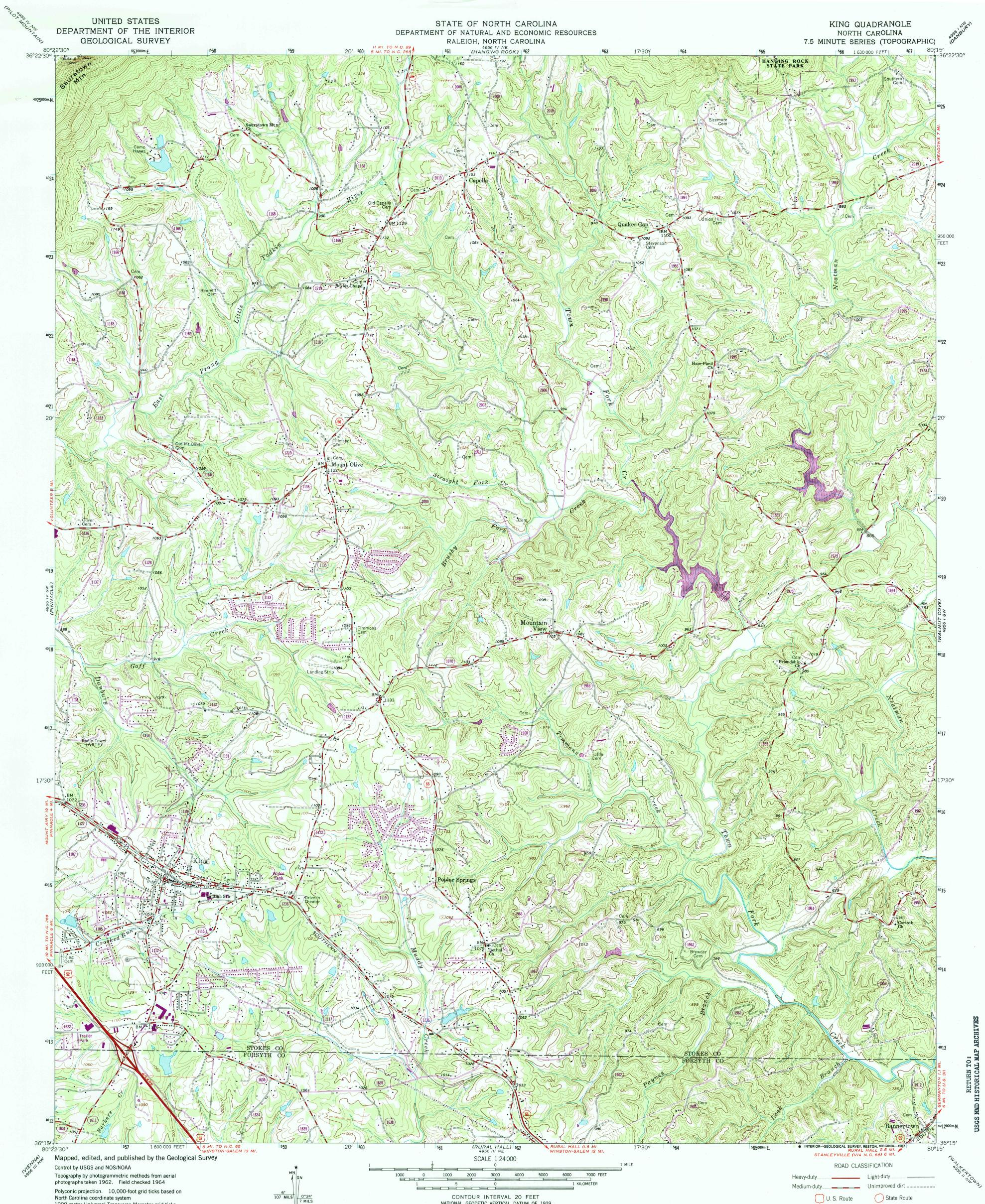
North Carolina coordinate system 1000-meter Universal Transverse Mercator grid ticks, zone 17, shown in blue 1927 North American Datum To place on the predicted North American Datum 1983 move the projection lines 10 meters south and 18 meters west as shown by dashed corner ticks
