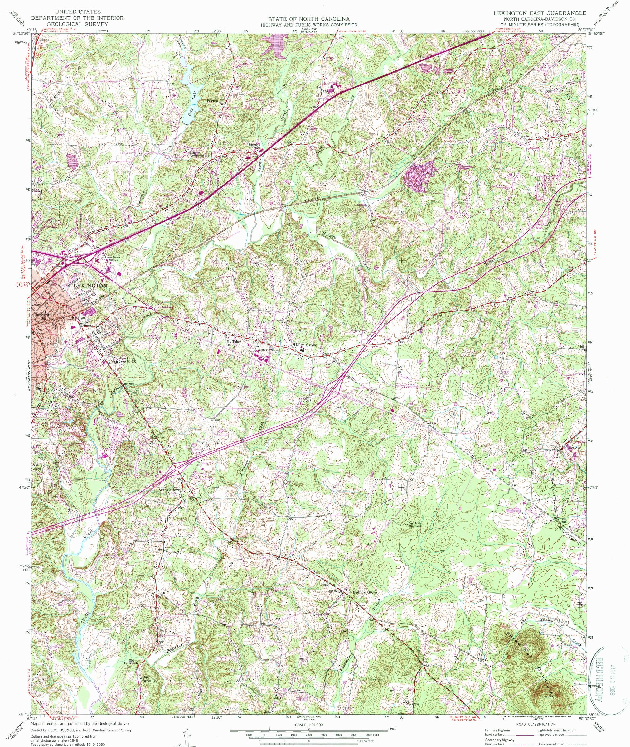
Polyconic projection. 1927 North American datum 10,000-foot grid based on North Carolina coordinate system 1000-metre Universal Transverse Mercator grid ticks, zone 17, shown in blue To place on the predicted North American Datum 1983 move the projection lines 10 meters south and 19 meters west as shown by dashed corner ticks 107 MILS 0°29' 9 MILS
