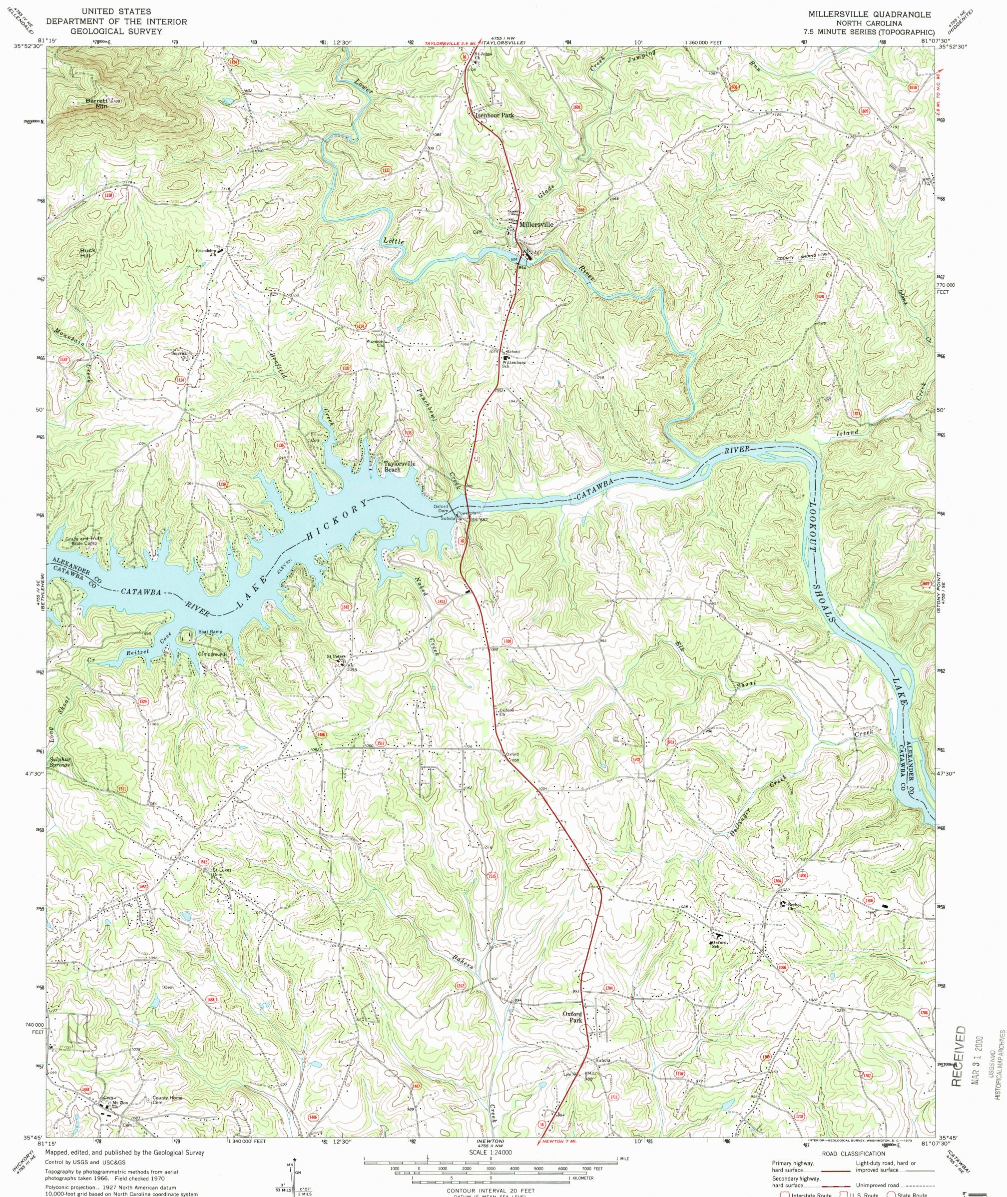
10,000-foot grid based on North Carolina coordinate system 1000-meter Universal Transverse Mercator grid ticks, zone 17, shown in blue
