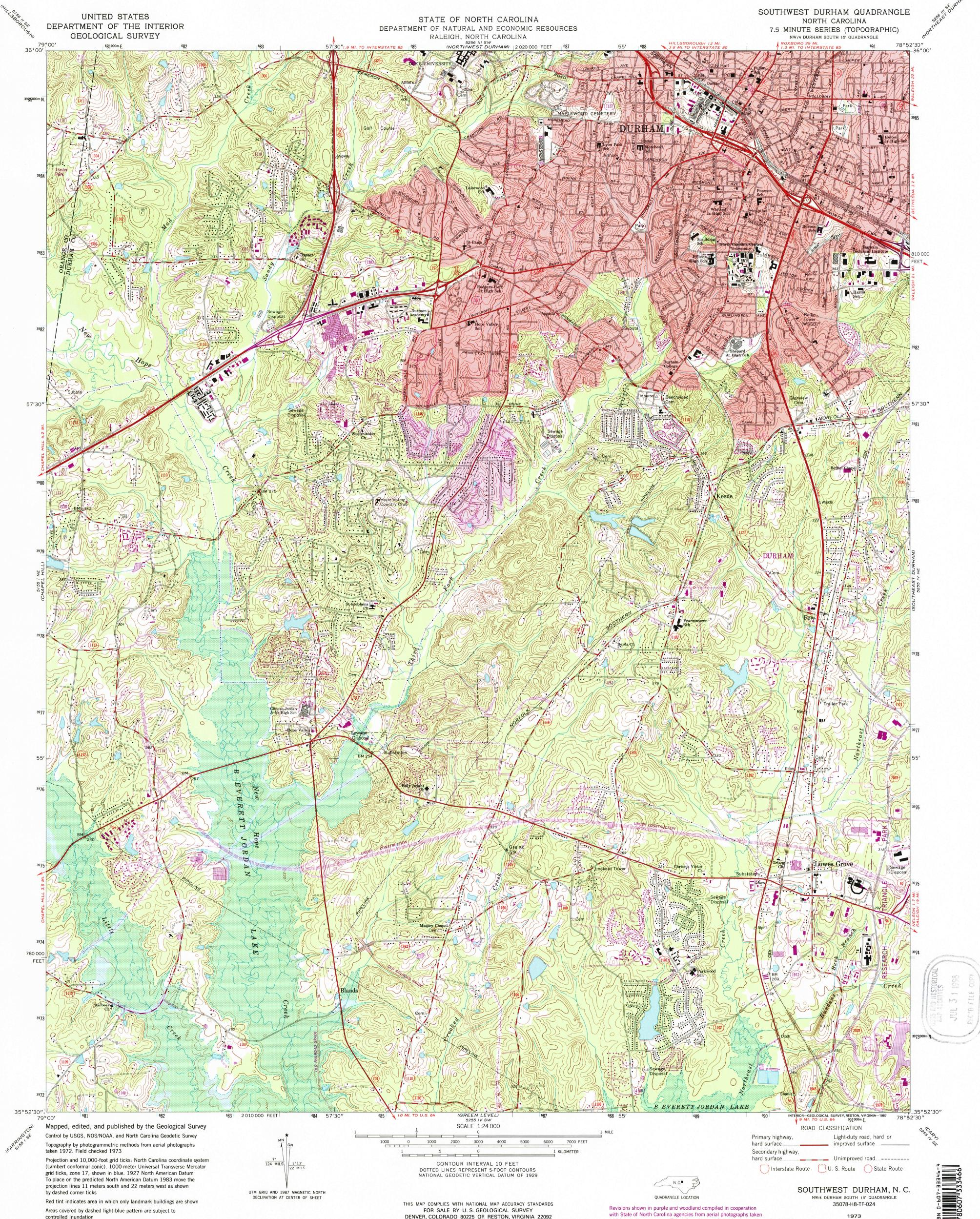
(Lambert conformal conic). 1000-meter Universal Transverse Mercator grid ticks, zone 17, shown in blue. 1927 North American Datum To place on the predicted North American Datum 1983 move the projection lines 11 meters south and 22 meters west as shown by dashed corner ticks
