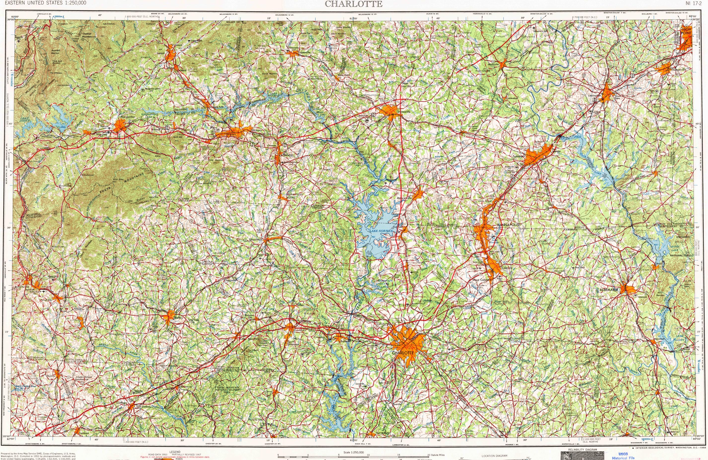
Prepared by the Army Map Service (AM), Corps of Engineers, U.S. Army, Washington, D.C. Compiled in 1953 by photogrammetric methods and from United States quadrangles, 1:24,000, 1:62,500, 1:100,000, and 1:125,000, 1905-50; county highway maps, 1943-49. Planimetric detail revised by photo-planimetric methods.Control by USGS and USCE. Map field checked 1953. Limited revision by U.S. Geological Survey 1967 1967.
