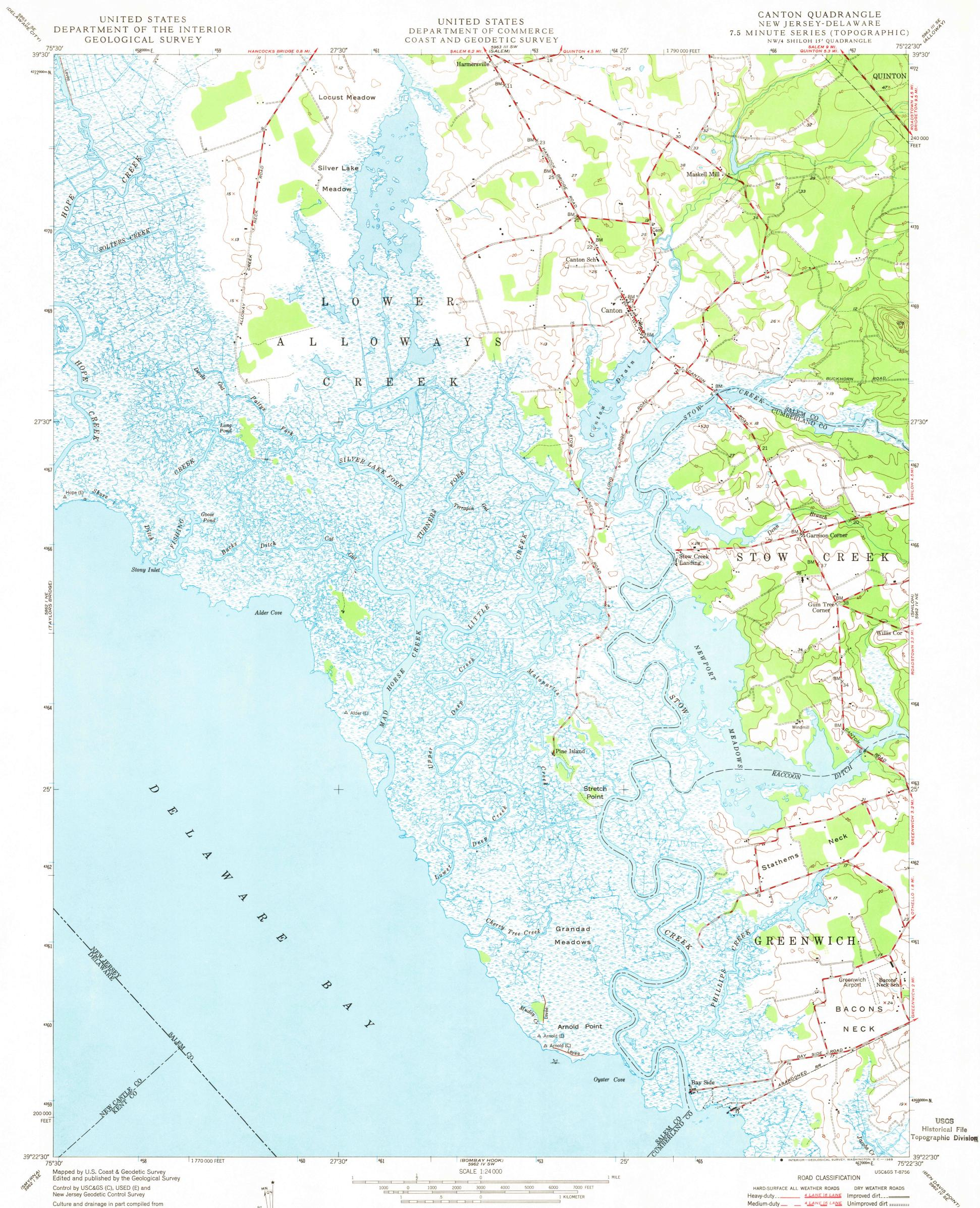
aerial photographs taken 1946 Topography by plane-table methods 1946 Field check 1948 Polyconic projection. 1927 North American datum 10,000-foot grids based New Jersey coordinate system No distinction is made between dwellings, barns, commercial and industrial buildings
