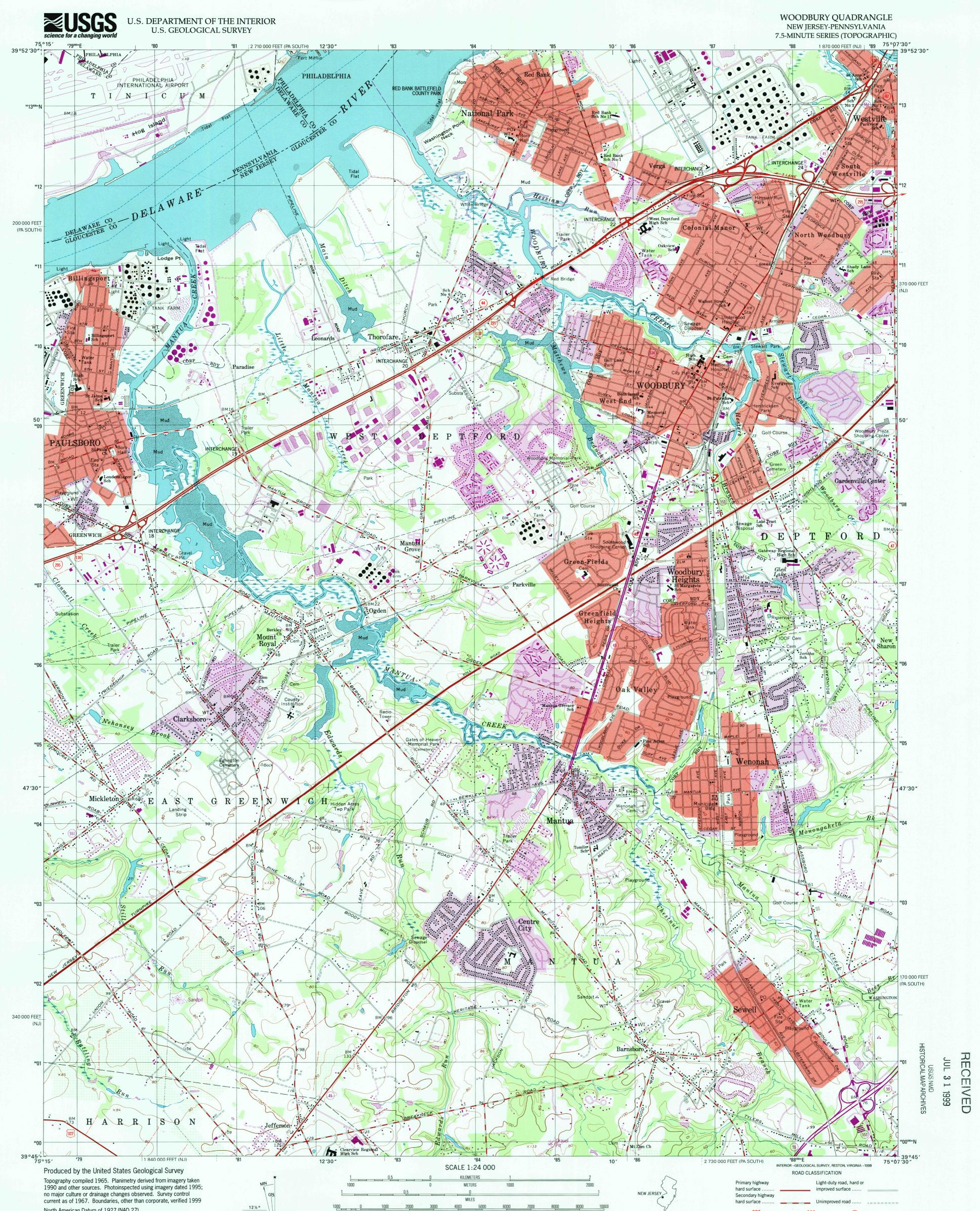
North American Datum of 1927 (NAD 27) Projection: New Jersey coordinate system (transverse Mercator) 10 000-foot ticks: New Jersey coordinate system and Pennsylvania coordinate system, south zone 1000-meter Universal Transverse Mercator grid, zone 18
