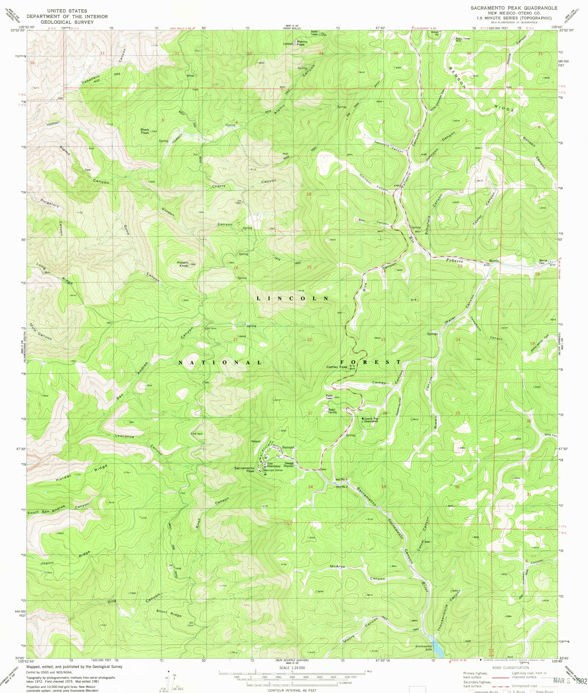
Projection and 10,000-foot grid ticks: New Mexico coordinate system, central zone (transverse Mercator) 1000-meter Universal Transverse Mercator grid, zone 13 1927 North-American datum To place on the predicted North American Datum 1983 move the projection lines 6 meters south and 50 meters east as shown by dashed corner ticks
