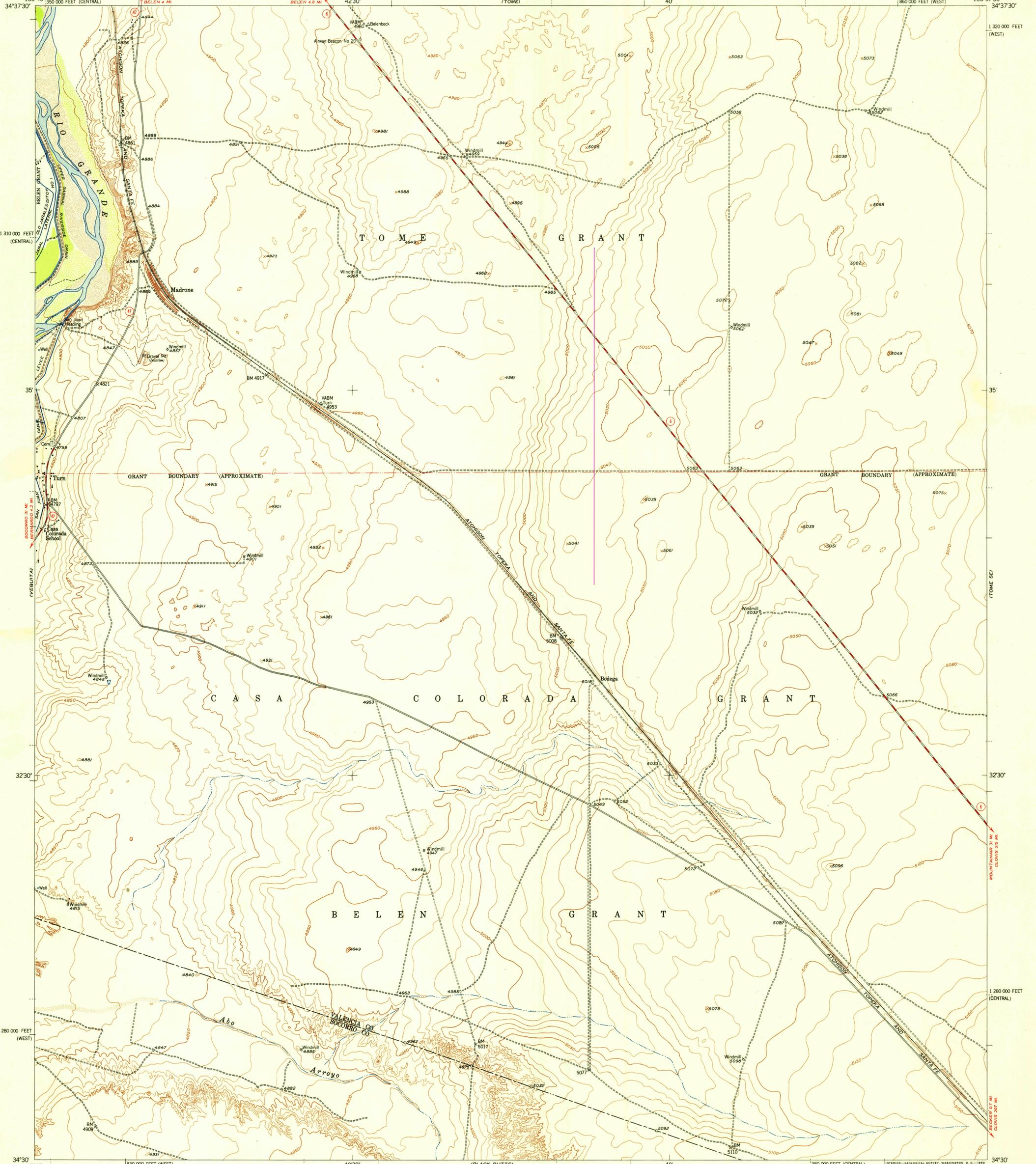
Mapped, edited, and published by the Geological Survey Control by USGS and USC&GS Topography from aerial photographs by multiplex methods and plane-table surveys 1952. Aerial photographs taken 1947 Polyconic projection. 1927 North American datum 10,000-foot grid based on New Mexico coordinate system, west and central zones Parts of west boundary of Tomé Grant and east boundary of Belén Grant are omitted because of insufficient data
