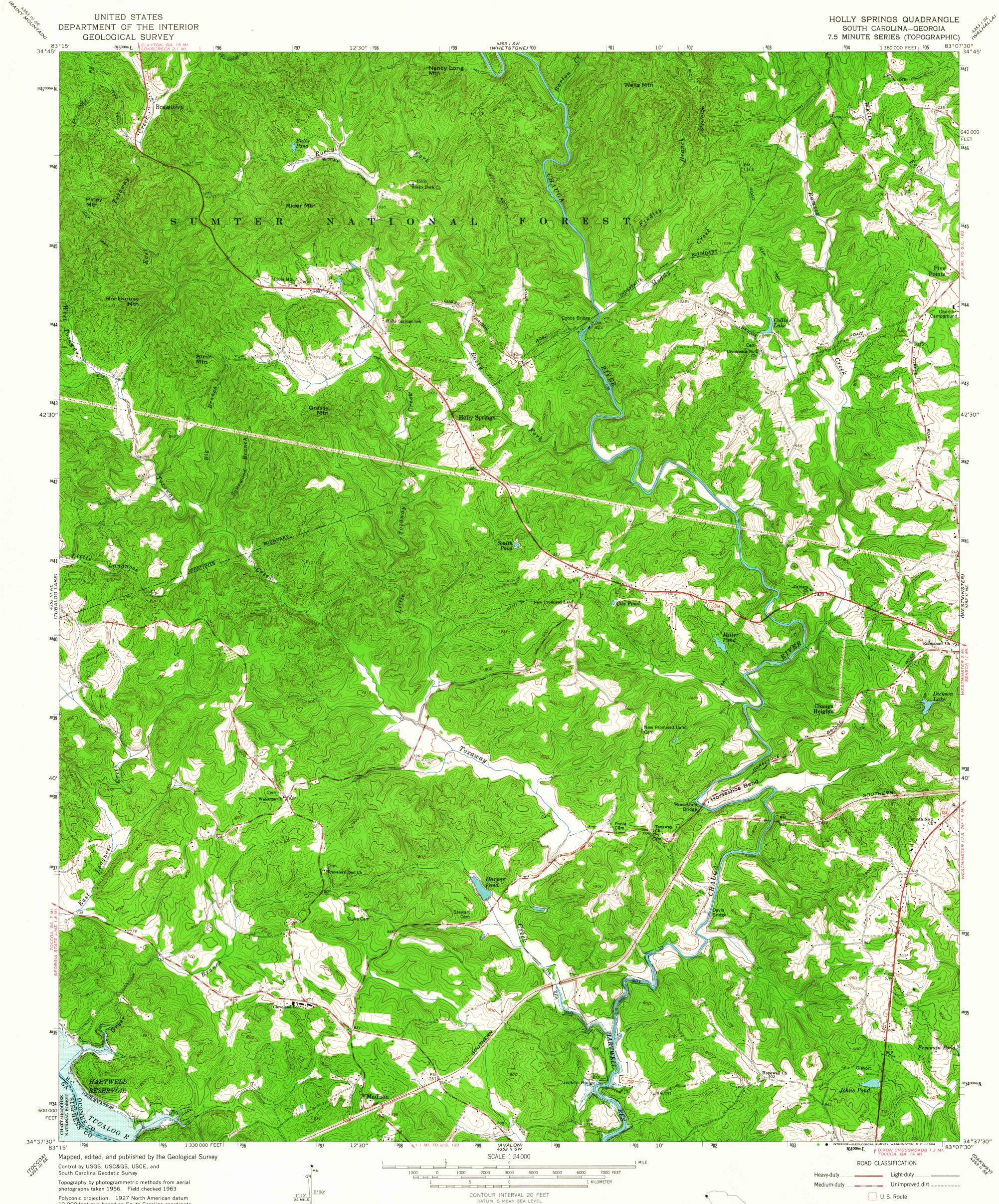
Polyconic projection. 1927 North American datum 10,000-foot grid based on South Carolina coordinate system, north zone 1000-meter Universal Transverse Mercator grid ticks, zone 17, shown in blue
