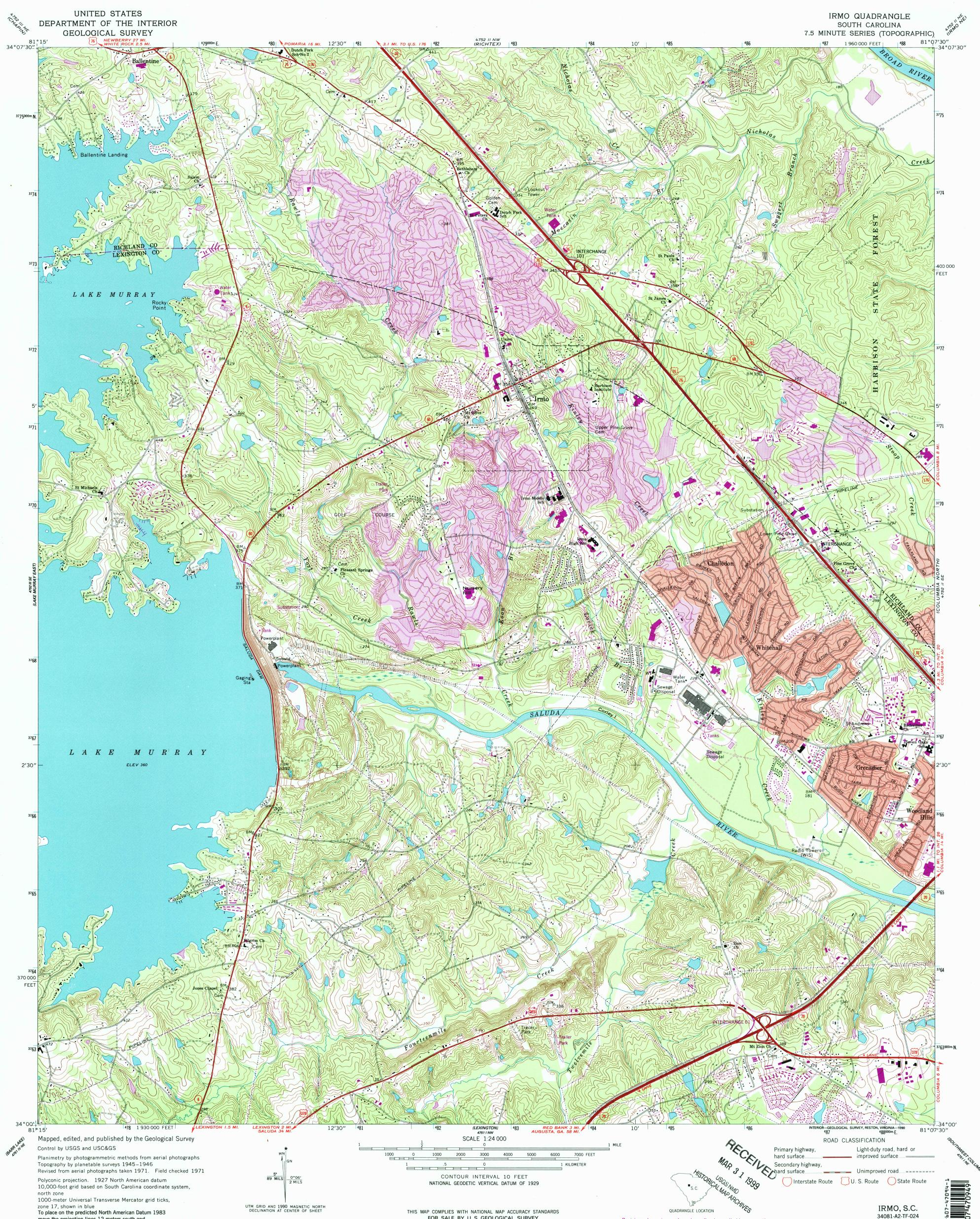
Polyconic projection. 1927 North American datum 10,000-foot grid based on South Carolina coordinate system, north zone 1000-meter Universal Transverse Mercator grid ticks, zone 17, shown in blue To place on the predicted North American Datum 1983 move the projection lines 12 meters south and 17 meters west as shown by dashed corner ticks
