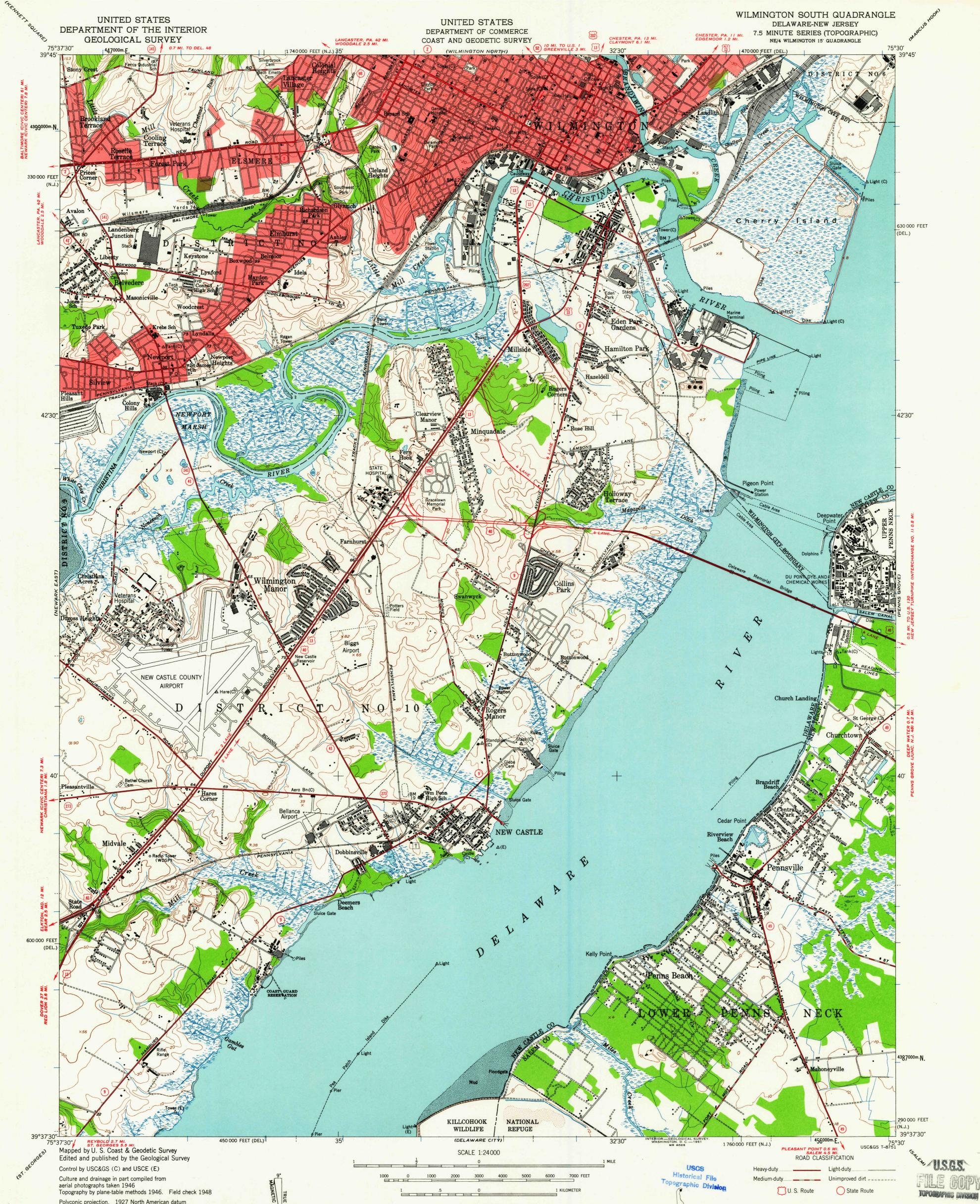
Topography by plane-table methods 1946. Field check 1948 Polyconic projection. 1927 North American datum 10,000-foot grids based on Delaware and New Jersey
