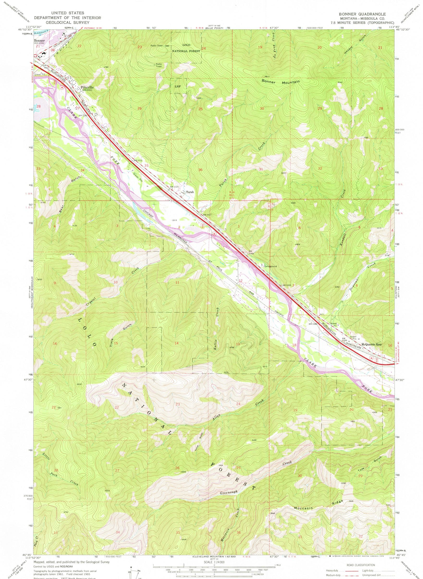
Polyconic projection. 1927 North American datum 10,000-foot grid based on Montana coordinate system, central zone 1000-meter Universal Transverse Mercator grid ticks, zone 12, shown in blue
