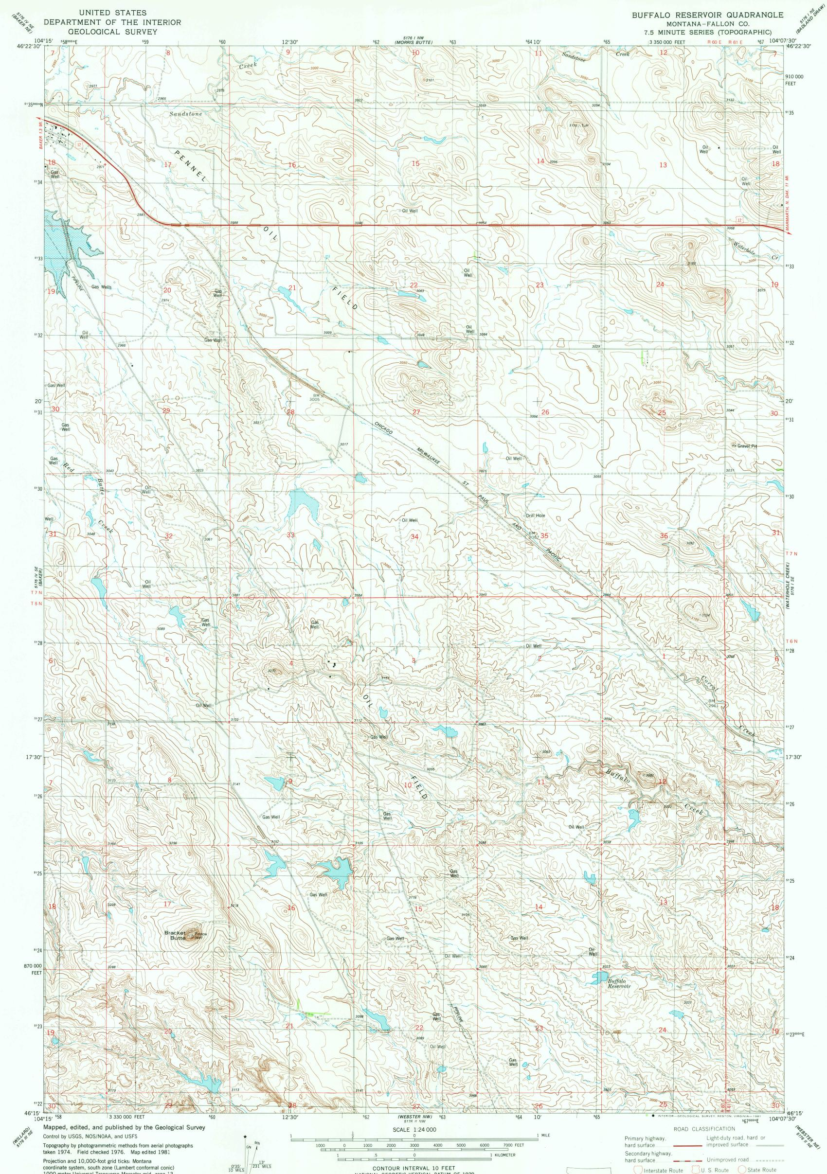
Projection and 10,000-foot grid ticks: Montana coordinate system, south zone (Lambert conformal conic) 1000-meter Universal Transverse Mercator grid, zone 13 1927 North American datum To place on the predicted North American Datum 1983 move the projection lines 4 meters north and 39 meters east as shown by dashed corner ticks Fine red dashed lines indicate selected fence lines Areas covered by dashed light-blue pattern
