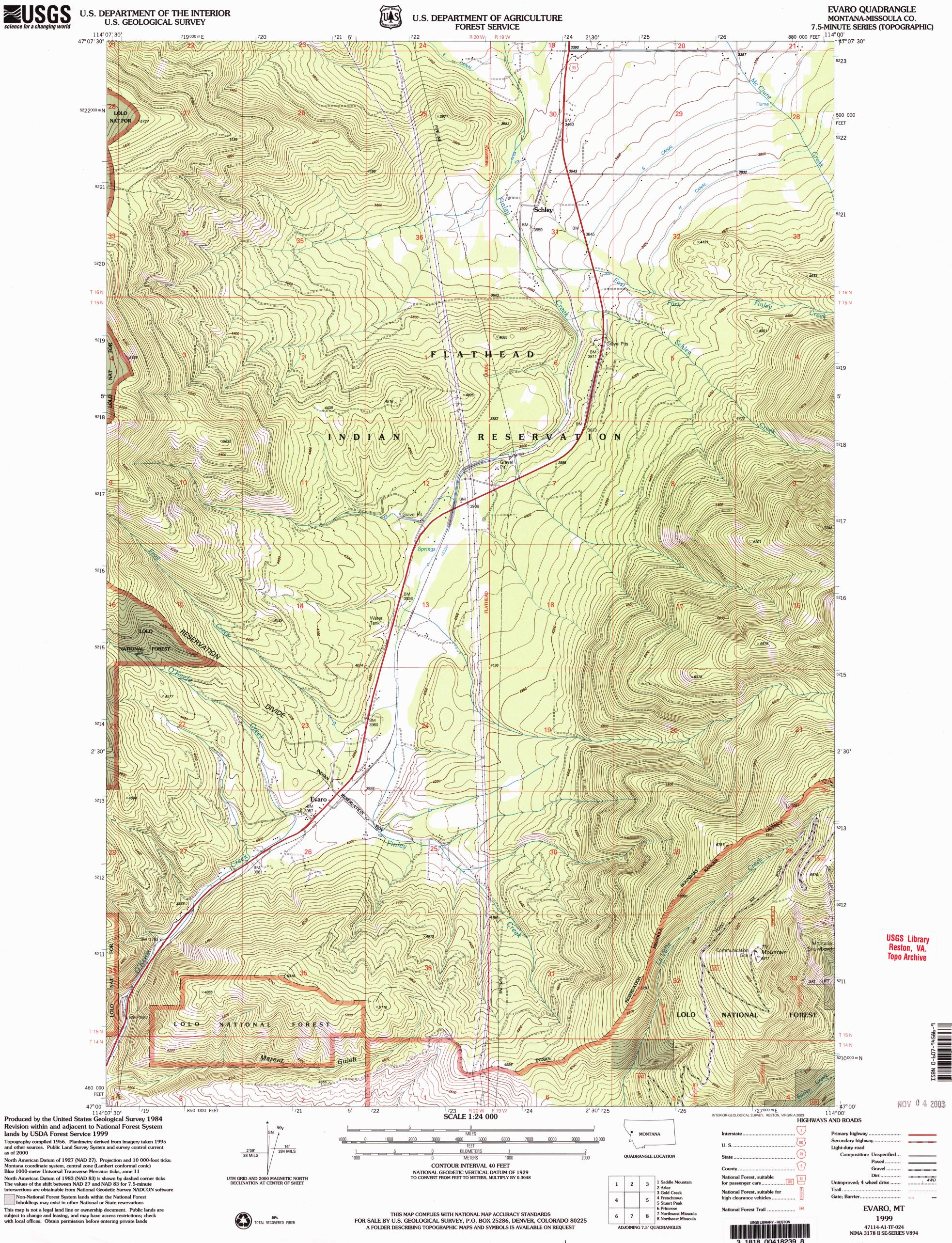
Montana coordinate system, central zone (Lambert conformal conic) Blue 1000-meter Universal Transverse Mercator ticks, zone 11 North American Datum of 1983 (NAD 83) is shown by dashed corner ticks The values of the shift between NAD 27 and NAD 83 for 7.5-minute intersections are obtainable from National Geodetic Survey NADCON software Non-National Forest System lands within the National Forest Inholdings may exist in other National or State reservations
