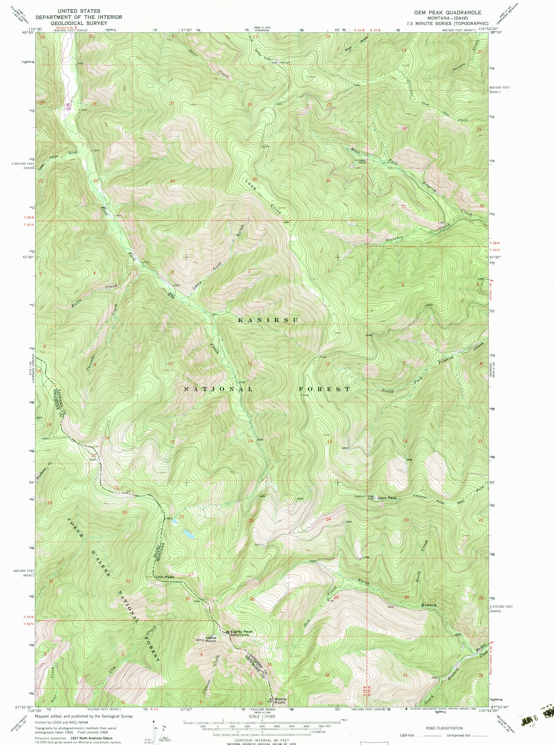
10,000-foot grids based on Montana coordinate system, central zone and Idaho coordinate system, west zone 1000-meter Universal Transverse Mercator grid ticks, zone 11, shown in blue
